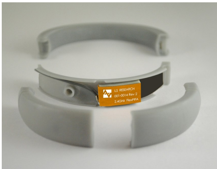
Figure 28: FlexPIFA integrated into bracelet
