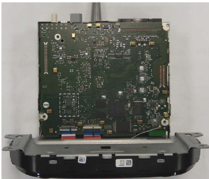
Figure5: VP2Refresh bottom view without bottom plate
