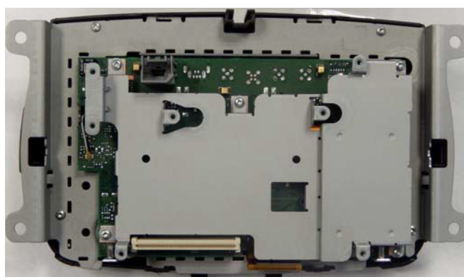
Figure7: VP2 Refresh FP backside view without power radio board
