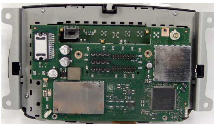
Figure6: VP2 Refresh FP backside view without fan and connector housing
