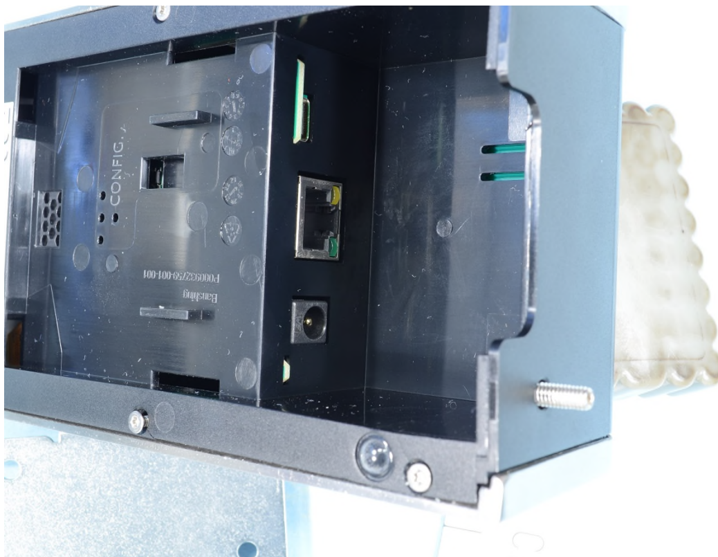
View of ports (Ethernet and DC)
