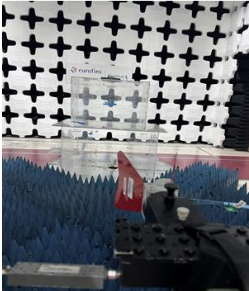
Figure 6. Radiated Spurious Emissions, (1 GHz – 18 GHz) Test Setup
