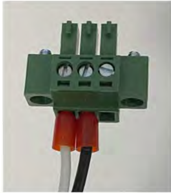
Basic Power Wiring (V+ and GND only)
