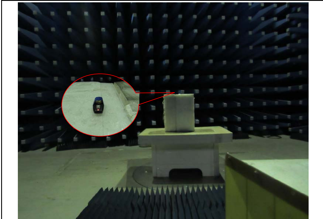
Radiated Spurious Emissions Test Setup Above 1GHz
