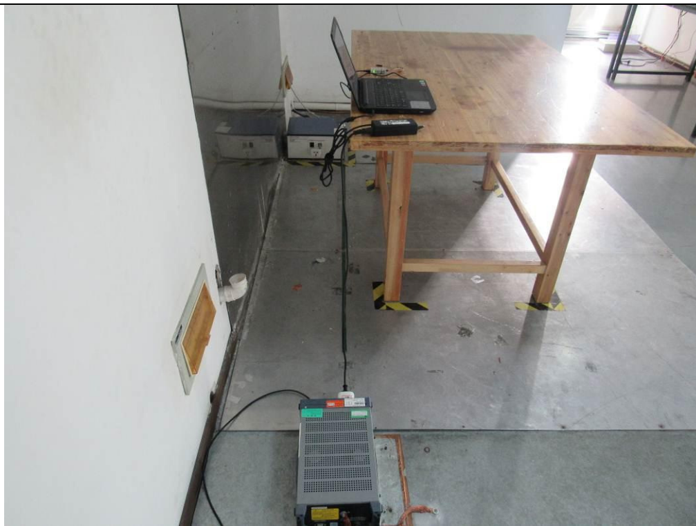
Conducted Emissions Setup Side View
