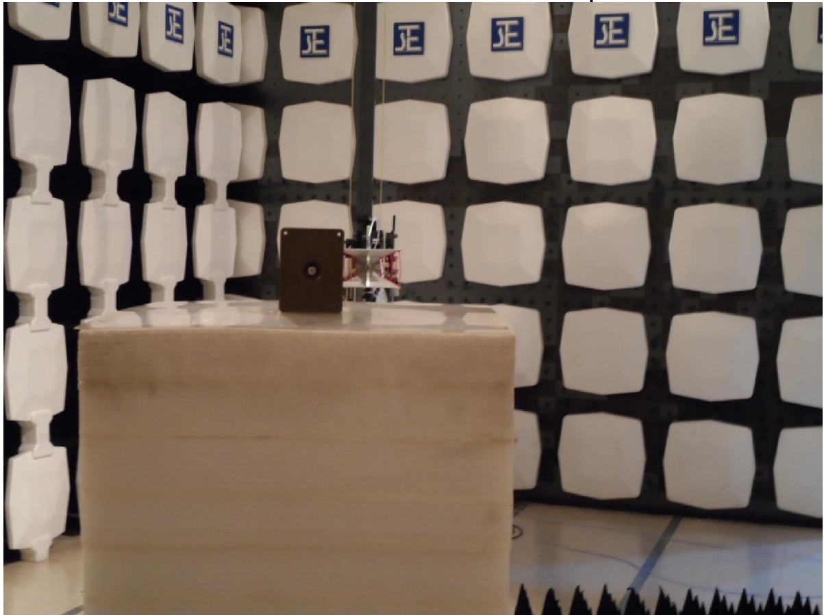
Measurement of Radiated Emission Test Set Up
