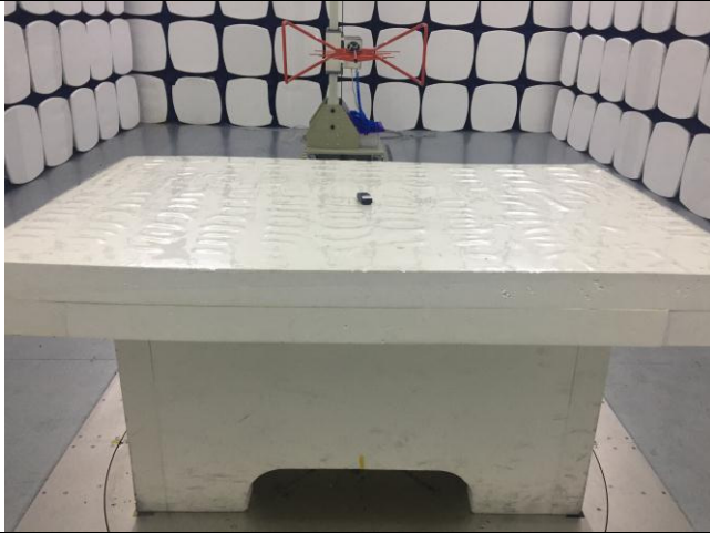
Radiated Spurious Emissions Test Setup Below 1GHz
