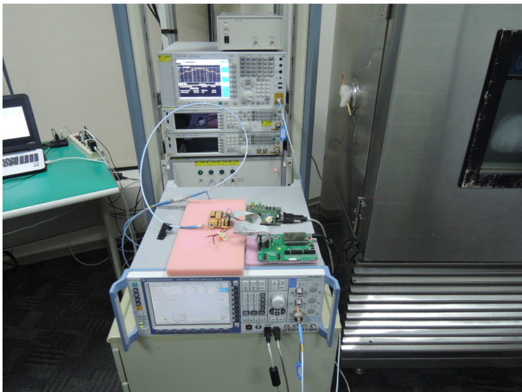
Photograph 5: Set-up for Conducted testing
