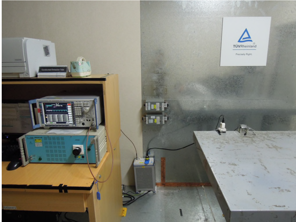
Photograph 8: Set-up for Mains Conducted testing (Back View)
