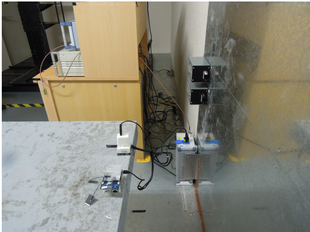
Photograph 8: Set-up for Mains Conducted testing (Back View)
