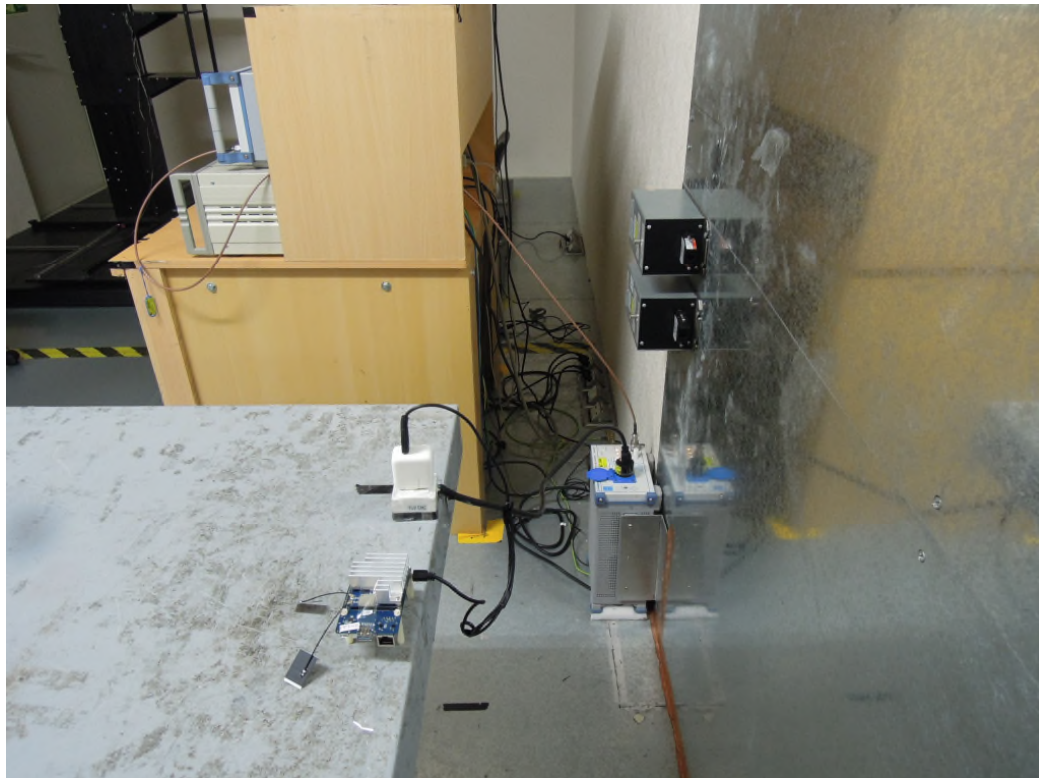
Photograph 6: Set-up for AC Mains Emissions (Back View)
