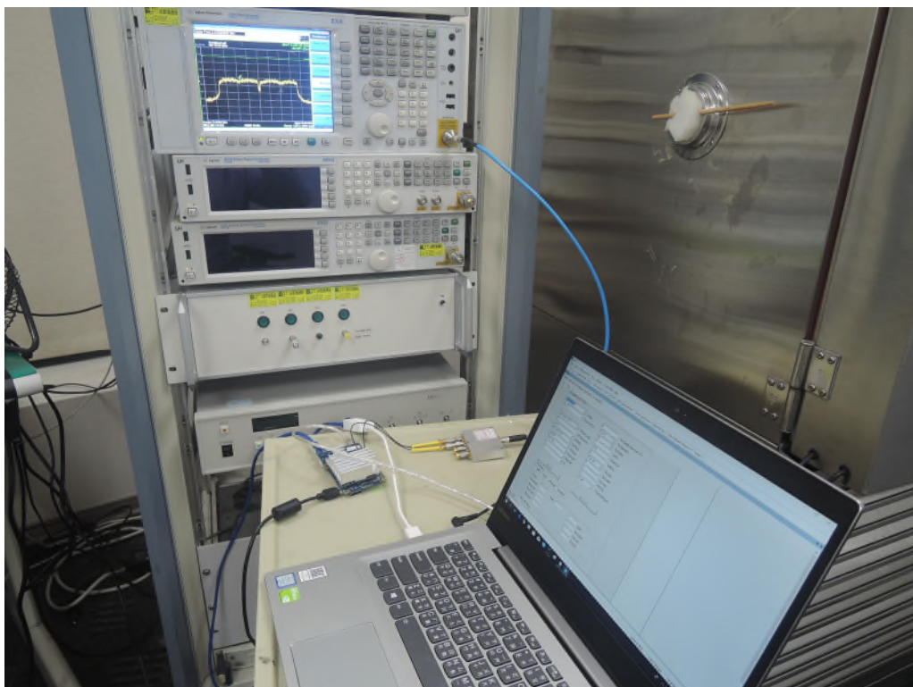
Photograph 4: Set-up for Conducted testing
