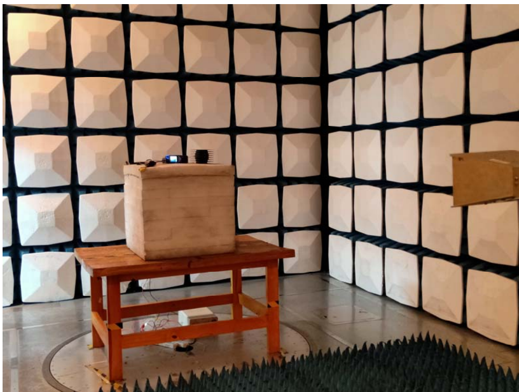
Radiated Emission Above 1GHz View
