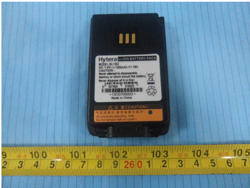
EUT – Battery View (1500mAh)
