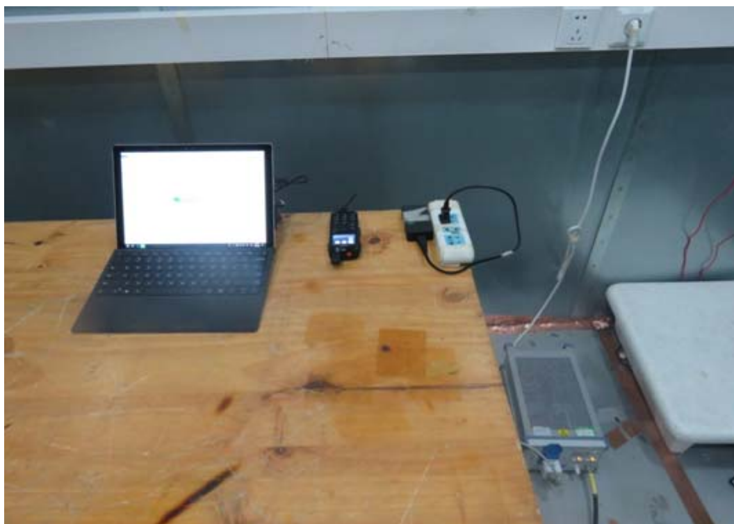
Picture 2 Conducted Emission Test Setup
