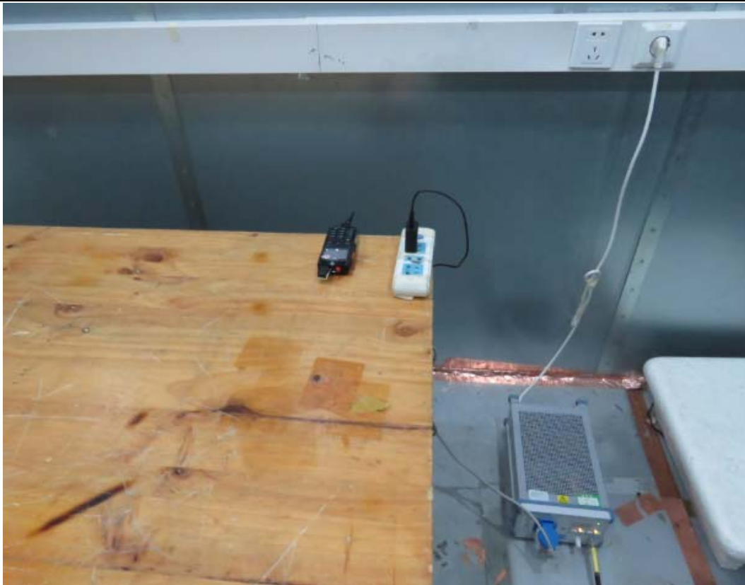
Picture 2 Conducted Emission Test Setup
