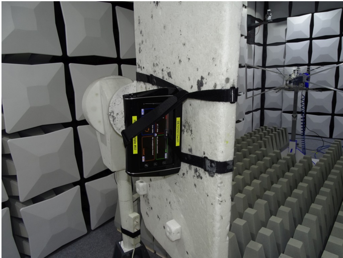
Photo 1: Test setup for radiated measurements (Enclosure, fully-anechoic chamber, 1-24 GHz intentional radiator §15)
