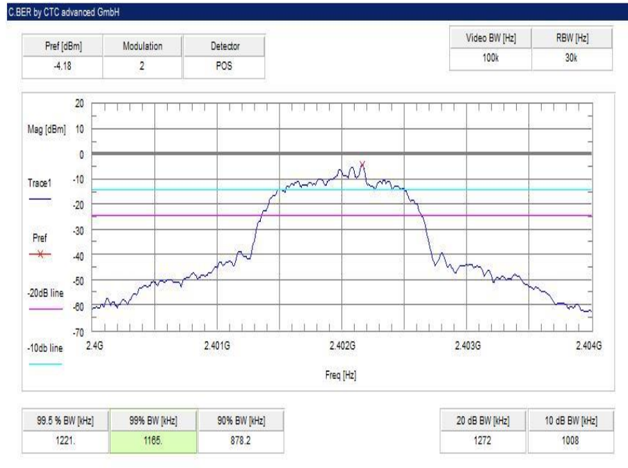
Plot 7: lowest channel – 2402 MHz, 8 DPSK modulation
