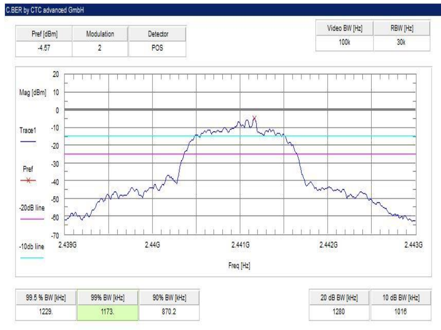
Plot 8: middle channel – 2441 MHz, 8 DPSK modulation
