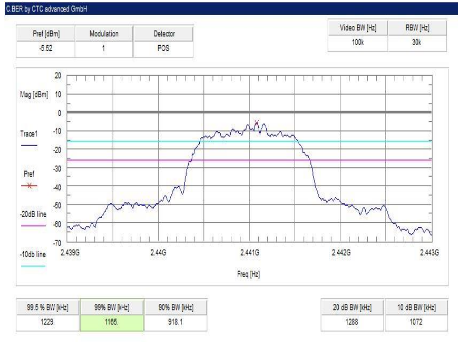
Plot 5: middle channel – 2441 MHz, Pi / DQPSK modulation
