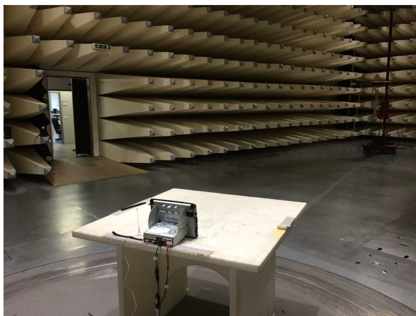
Photo 12 - RSE setup (30MHz-1GHz)
