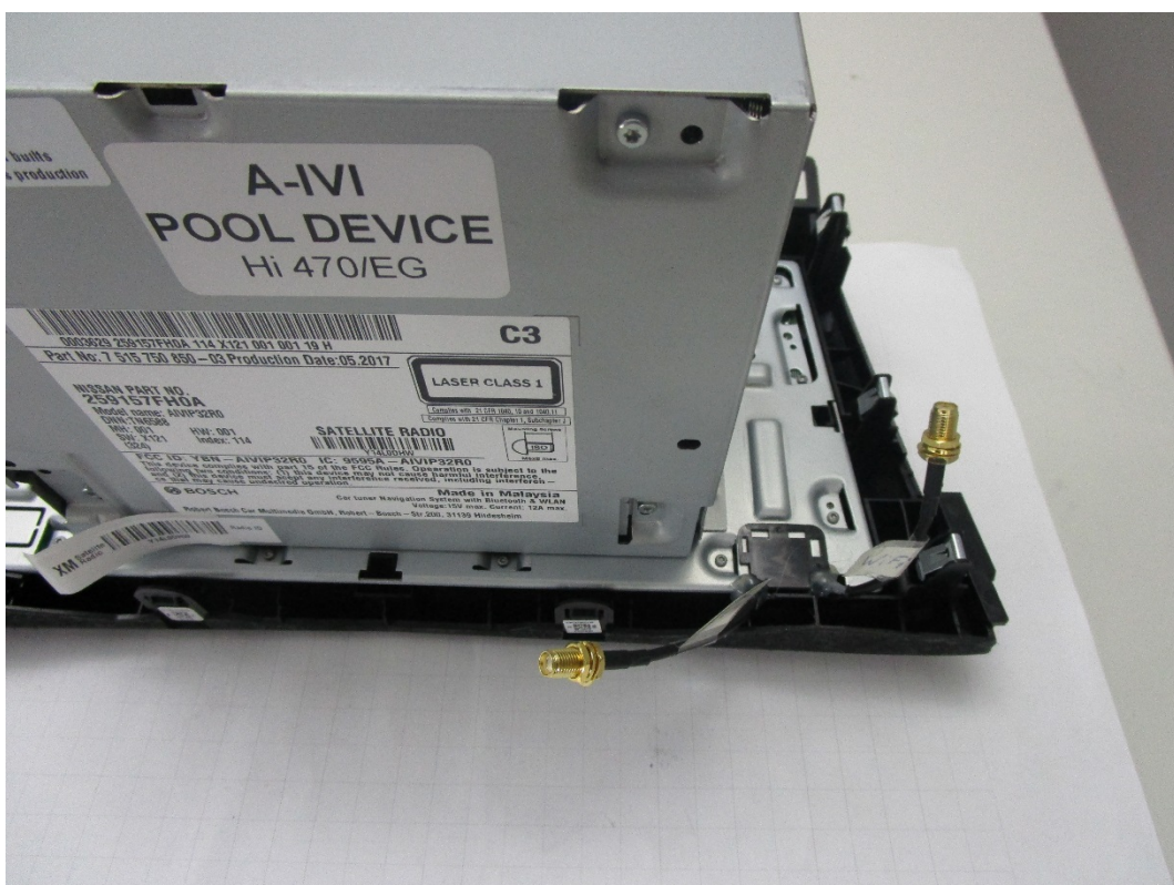
Photograph 9:AIVI – Top Side-Connector View
