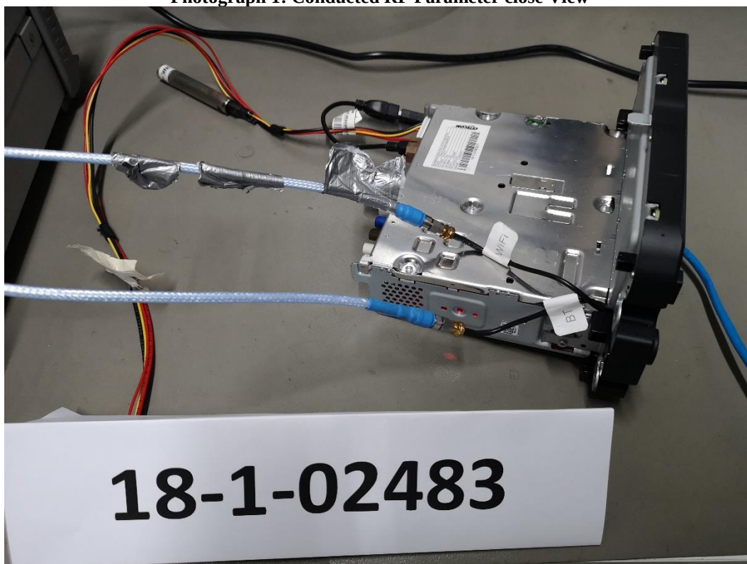
Photograph 2: Conducted RF Parameter close View
