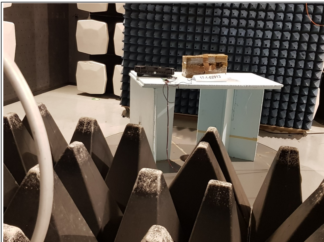
Photograph 1: Magnetic fields measurement test set-up (overview)
