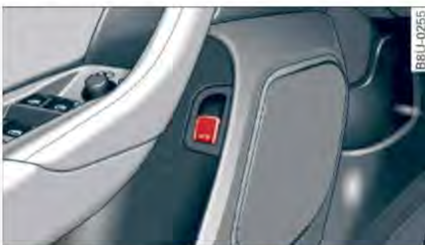
Fig. 22 Driver's door: opening the luggage compartment lid
