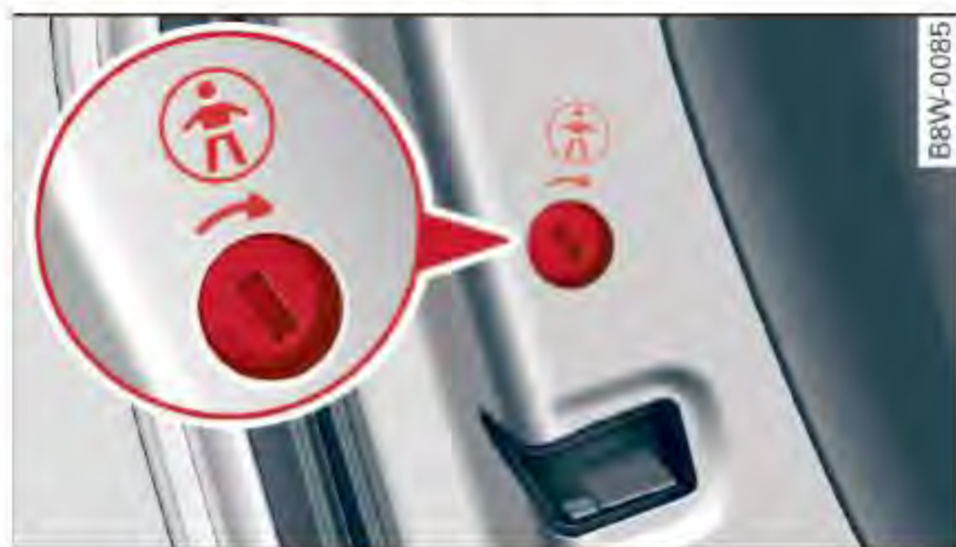
Fig. 27 Rear door: child safety lock
