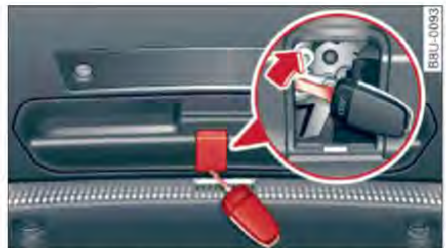
Fig. 25 Luggage compartment lid emergency release
