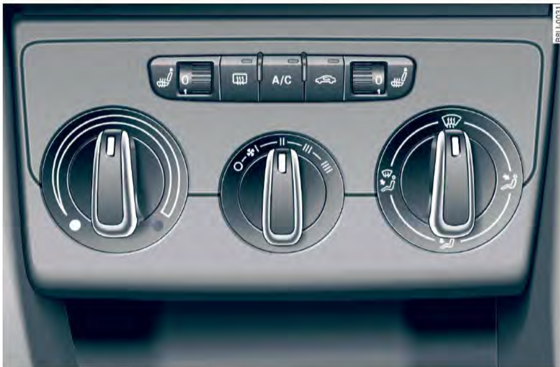
Fig. 65 Manual climate control system controls
