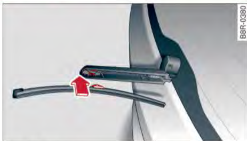
Fig. 42 Rear window wiper: removing the wiper blade
