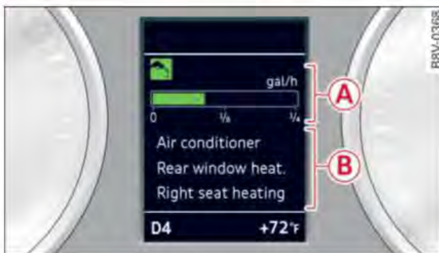
Fig. 11 Instrument cluster: energy consumers
