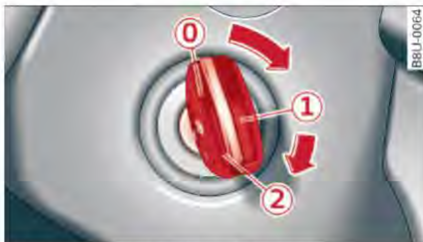
Fig. 68 Ignition lock: position of the ignition key
