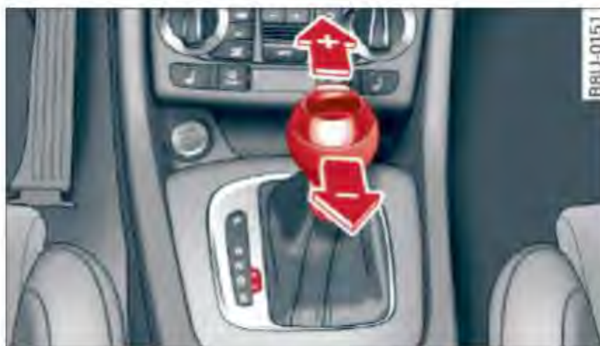
Fig. 74 Center console: shifting manually with the selector lever
