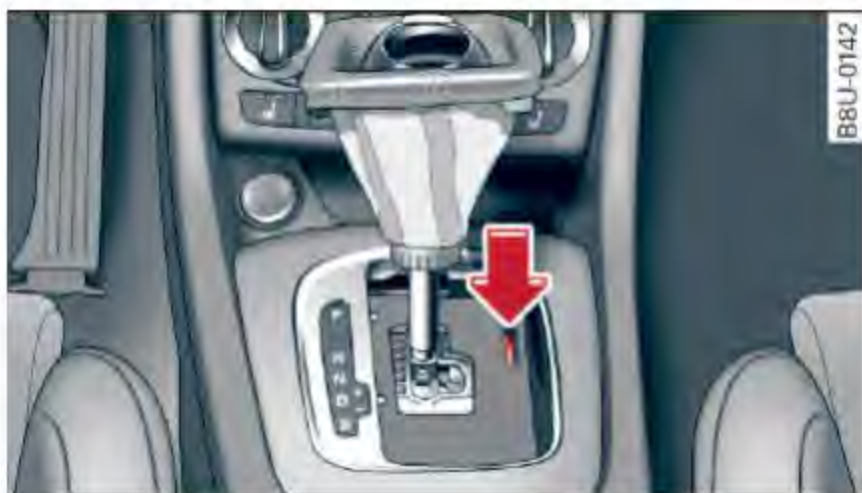
Fig. 77 Selector lever: emergency release
