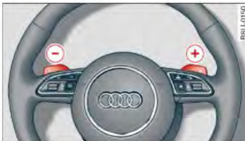
Fig. 75 Steering wheel: shifting manually with the shift paddles*
