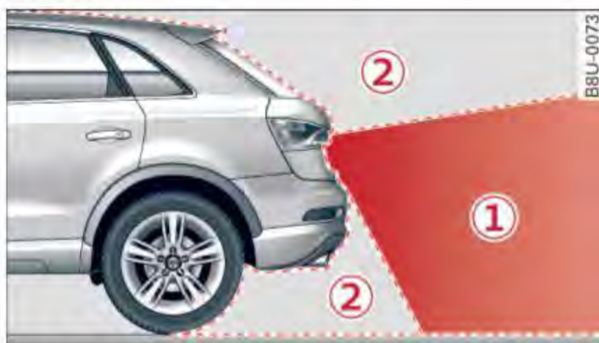
Fig. 90 Area covered ① and area not covered ② by the rearview camera.
