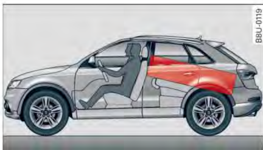
Fig. 100 Safe load positioning: place heavy objects as low and as far forward as possible.
