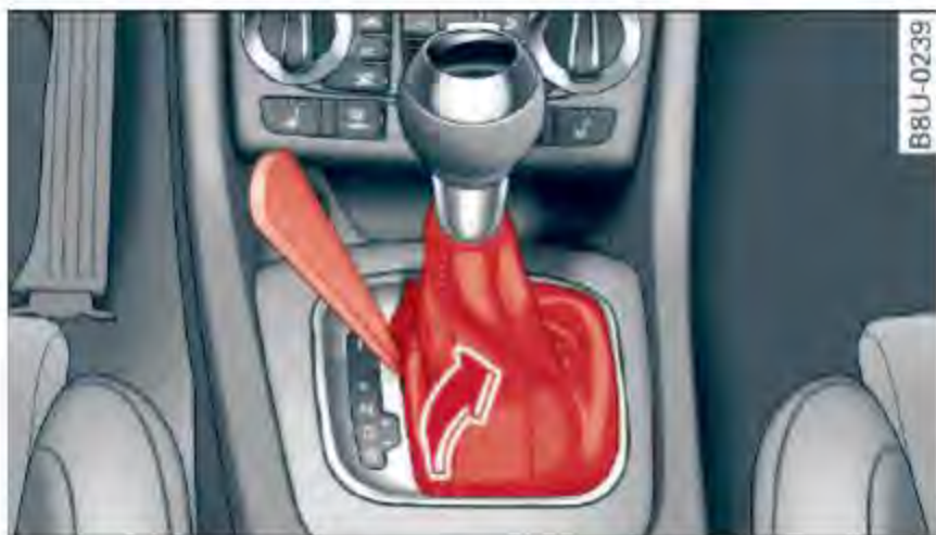
Fig. 76 Selector lever: removing the cover
