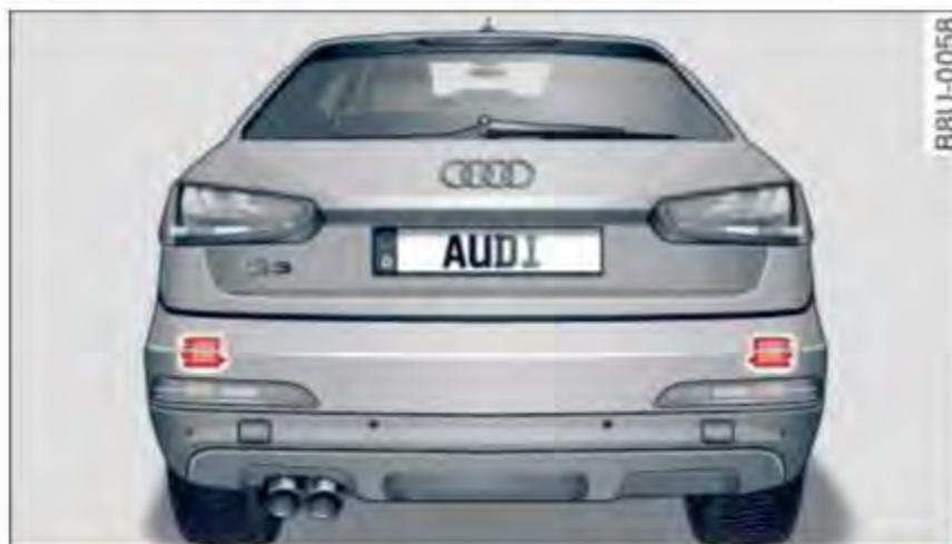
Fig. 82 Rear of the vehicle: position of the sensors
