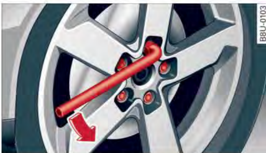
Fig. 151 Changing a wheel: loosening the wheel bolts
