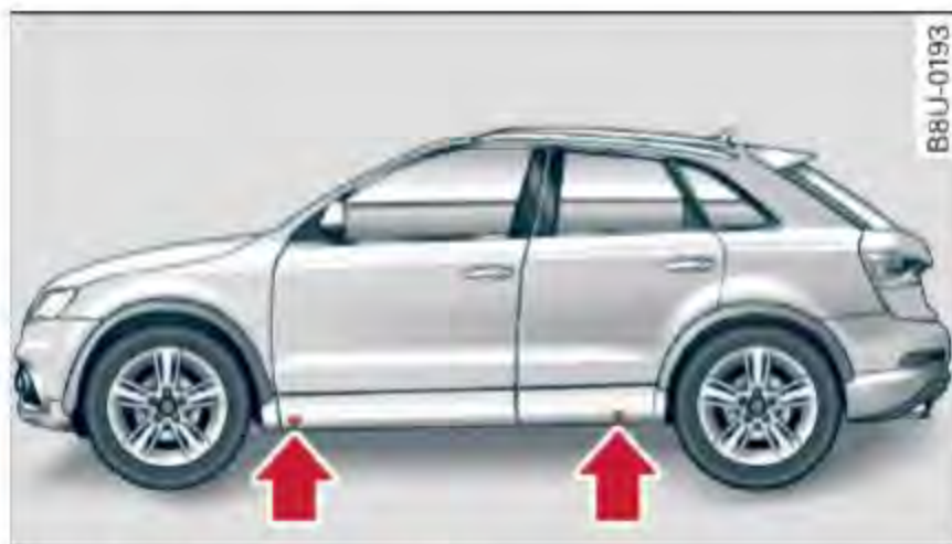
Fig. 152 Sill panels: markings
