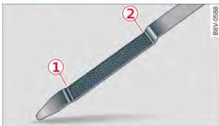
Fig. 138 Oil dipstick (example): checking the engine oil level
