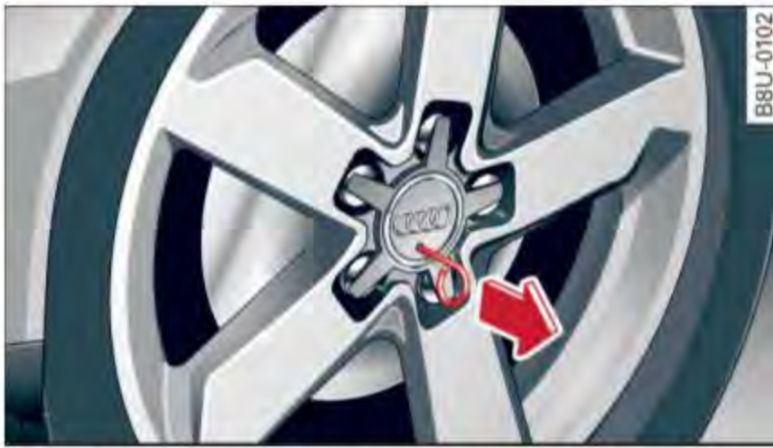
Fig. 149 Changing a wheel: removing the wheel cover
