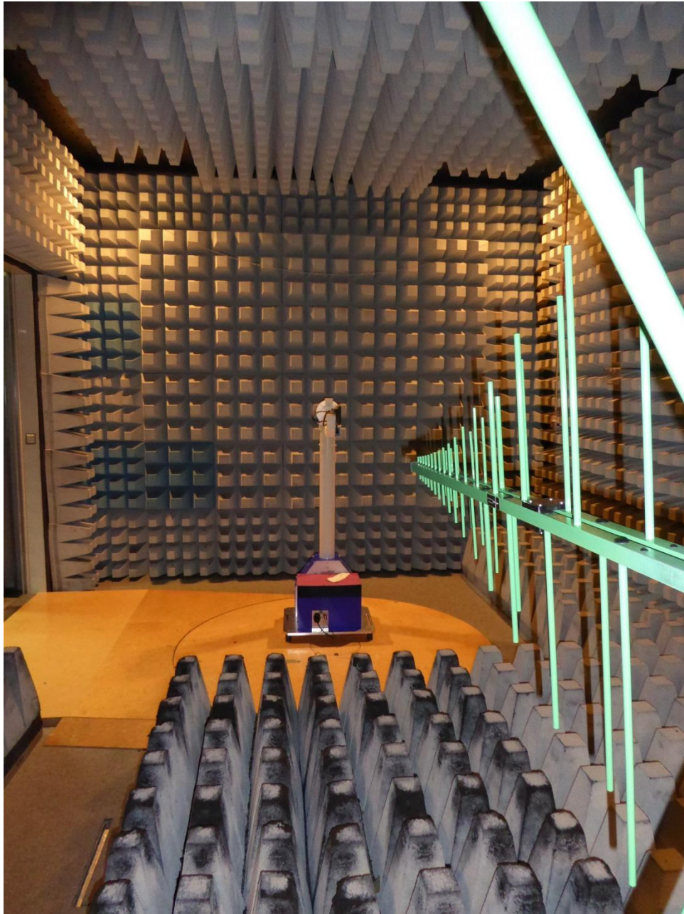
162097_03.jpg: Test setup fully anechoic chamber
