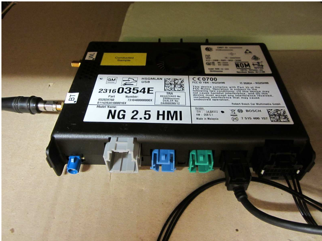
Photo 6: Test setup for conducted measurements
