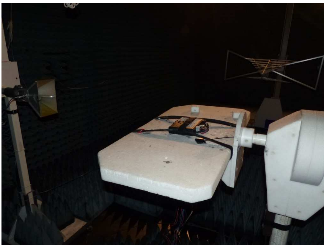
Photo 4: Test setup for radiated measurements (above 1 GHz)
