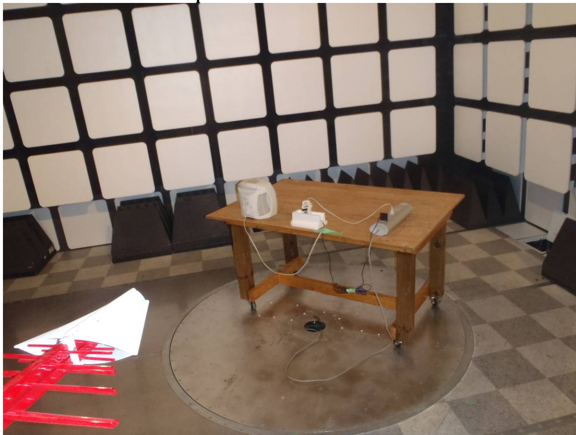
Radiated Emission Test Setup Photo #1:
