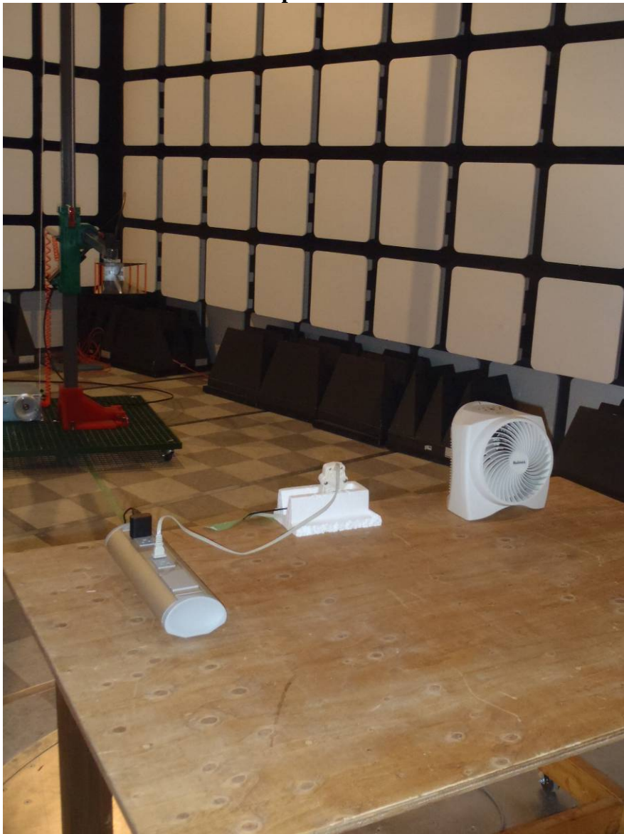
Radiated Emission Test Setup Photo #2:
