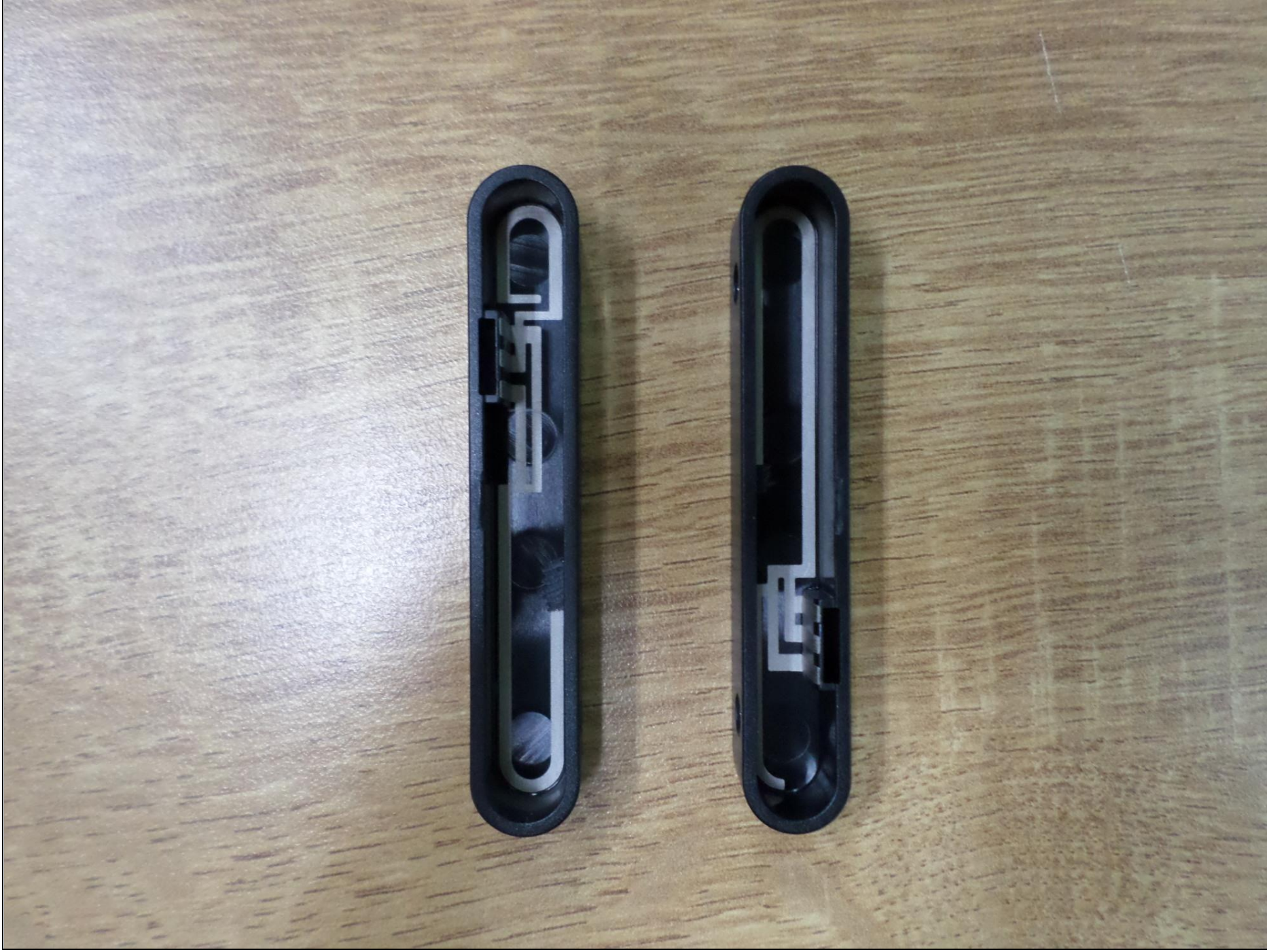
View of Antenna
