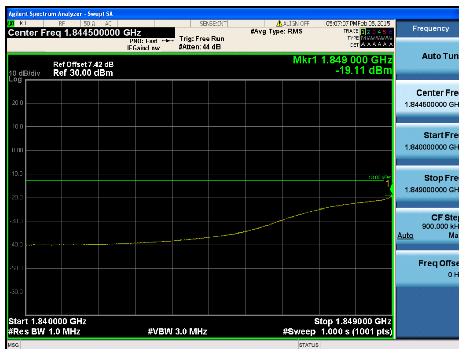
LTE Band 25 / 10MHz / QPSK - RB Size/Offset (25/0)
