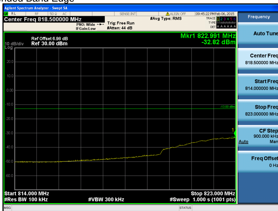
LTE Band 26 / 10MHz / QPSK - RB Size/Offset (25/0)
