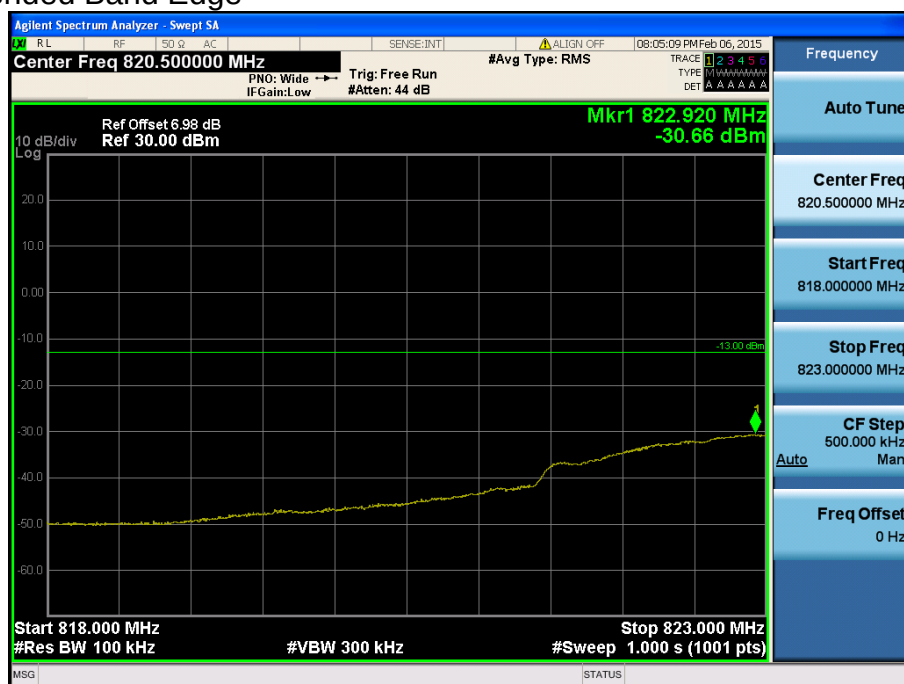
LTE Band 26 / 3MHz / QPSK - RB Size/Offset (1/14)
