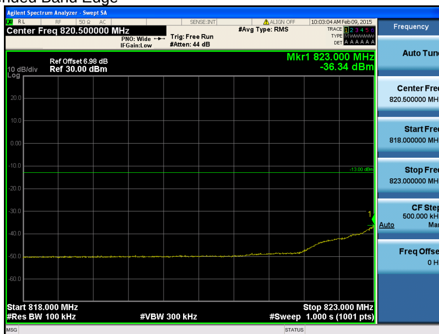
LTE Band 26 / 1.4MHz / 16QAM - RB Size/Offset (1/3)
