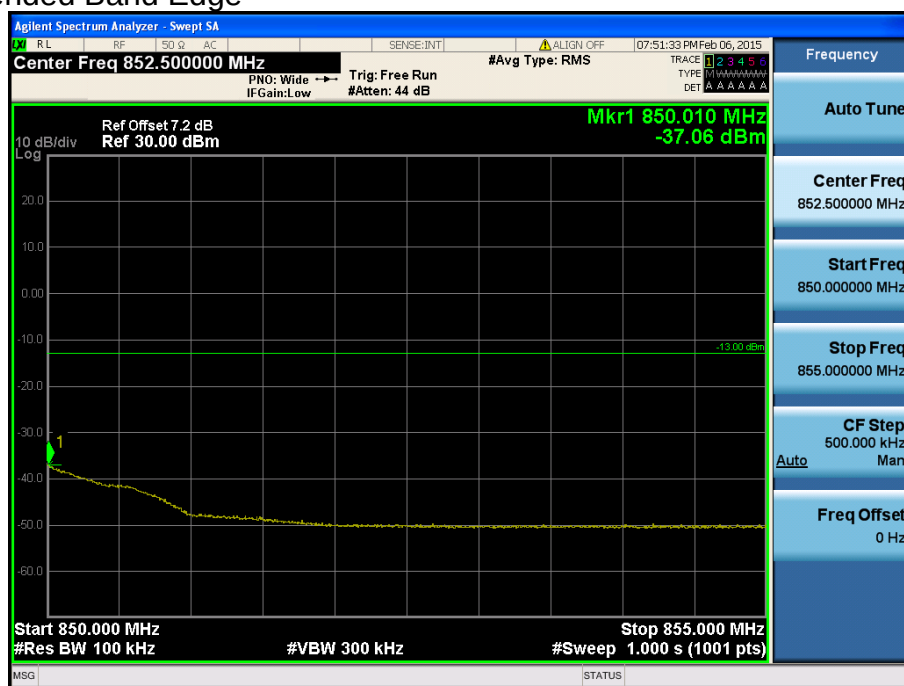
LTE Band 26 / 1.4MHz / QPSK - RB Size/Offset (6/0)
