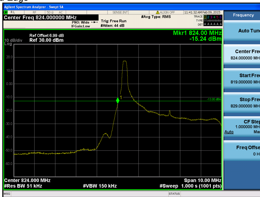
LTE Band 26 / 5MHz / 16QAM - RB Size/Offset (1/0)
