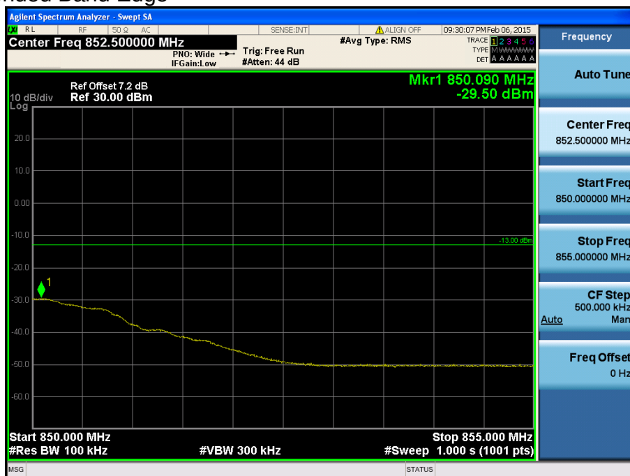
LTE Band 26 / 5MHz / QPSK - RB Size/Offset (12/13)
