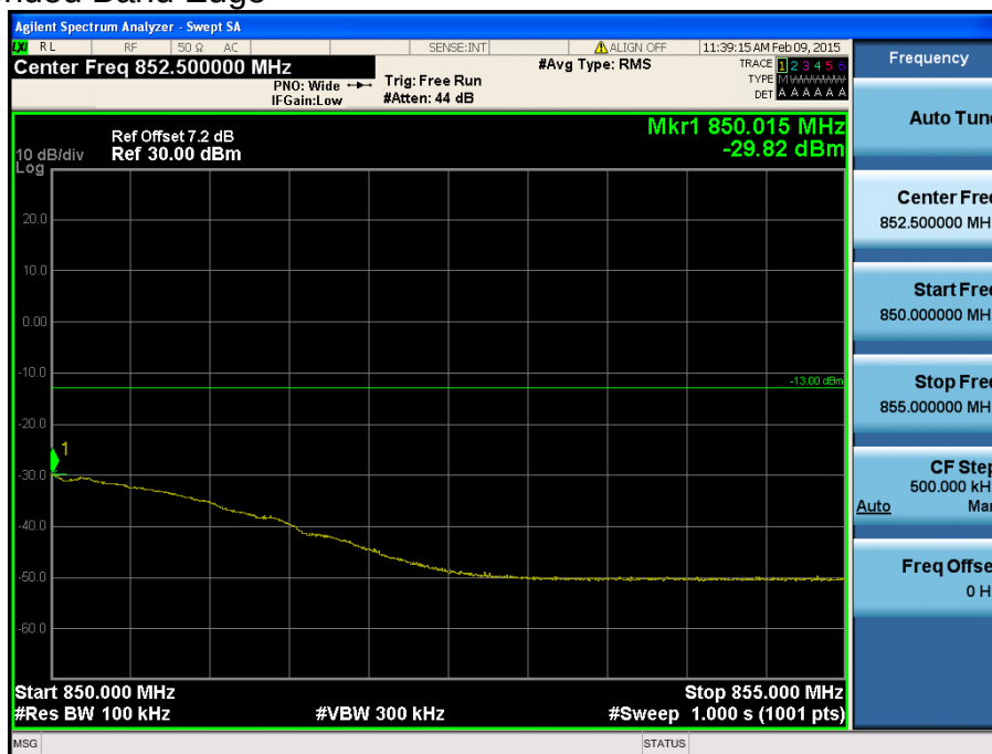
LTE Band 26 / 3MHz / 16QAM - RB Size/Offset (15/0)
