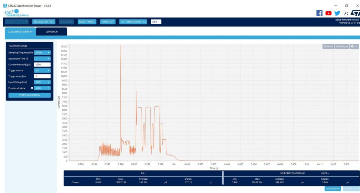
Figure 12. Example of current measurement with an external STLINK-V3PWR
