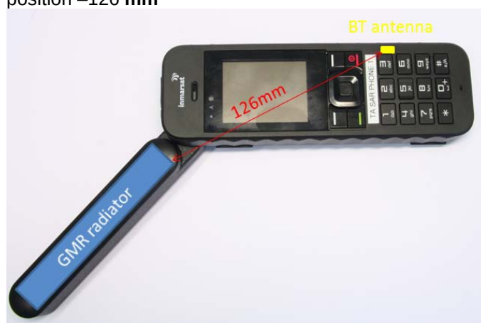
Antenna dimensions and separation distances
