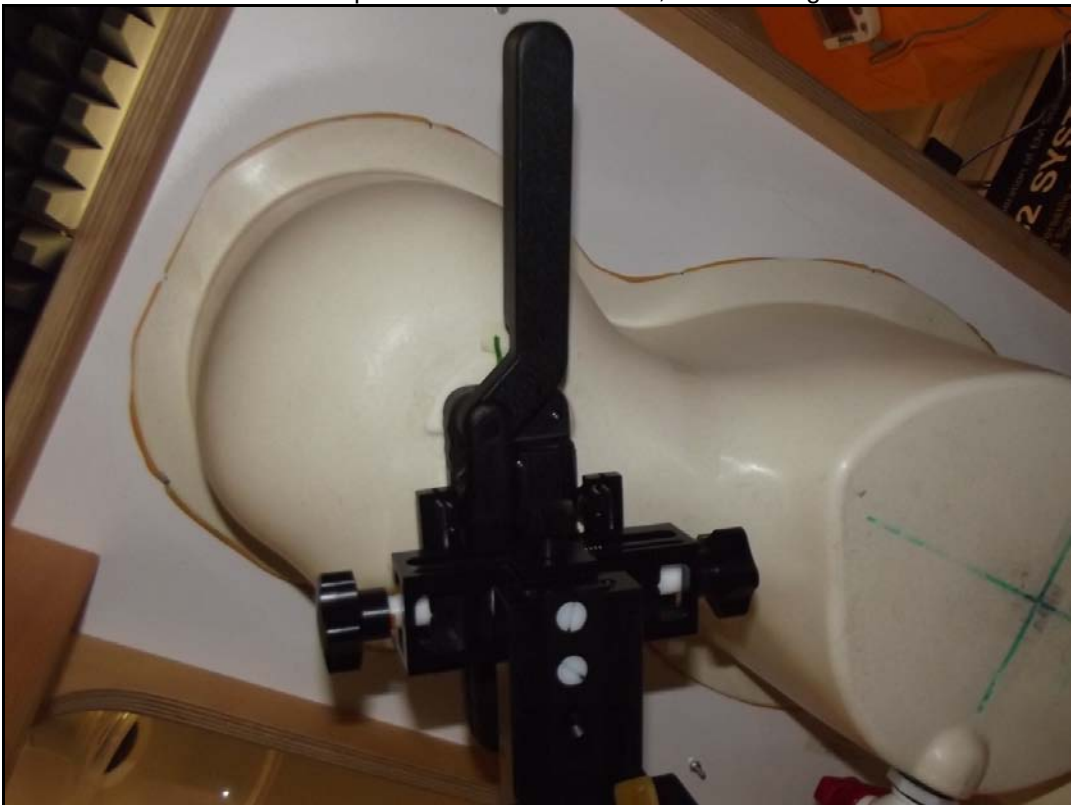
Photo 14: Test position left hand touched, antenna angle 180°
