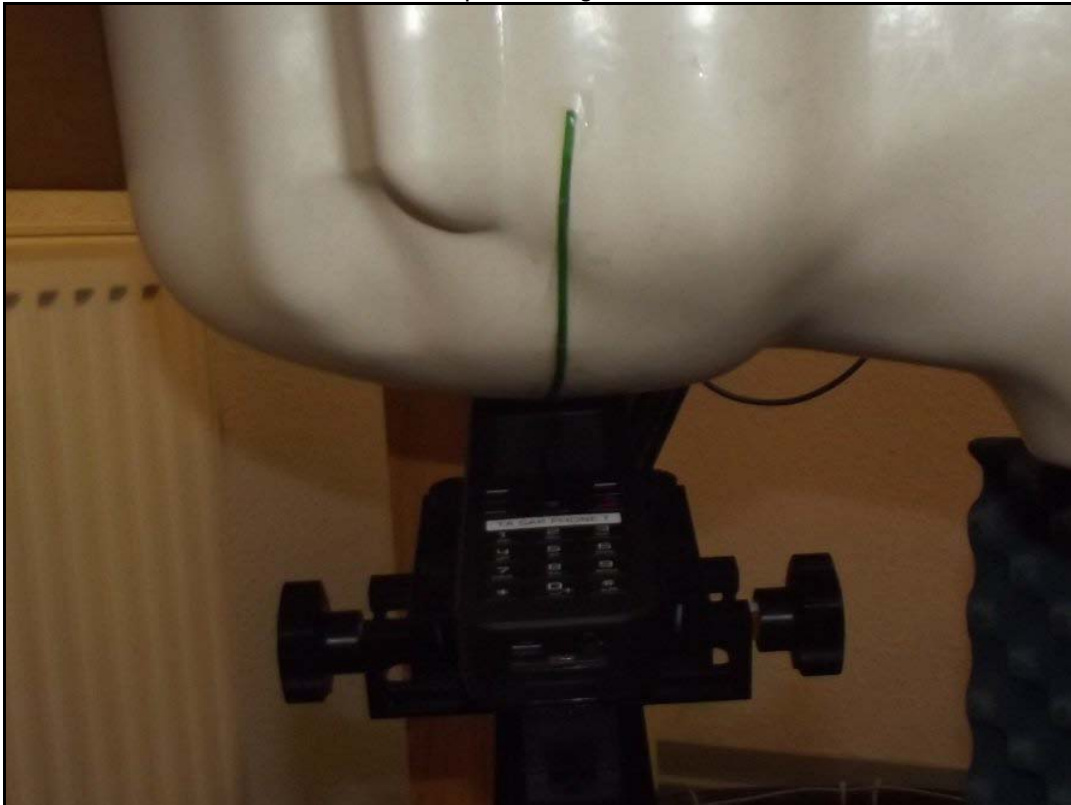
Photo 22: Test position right hand tilted 15°
