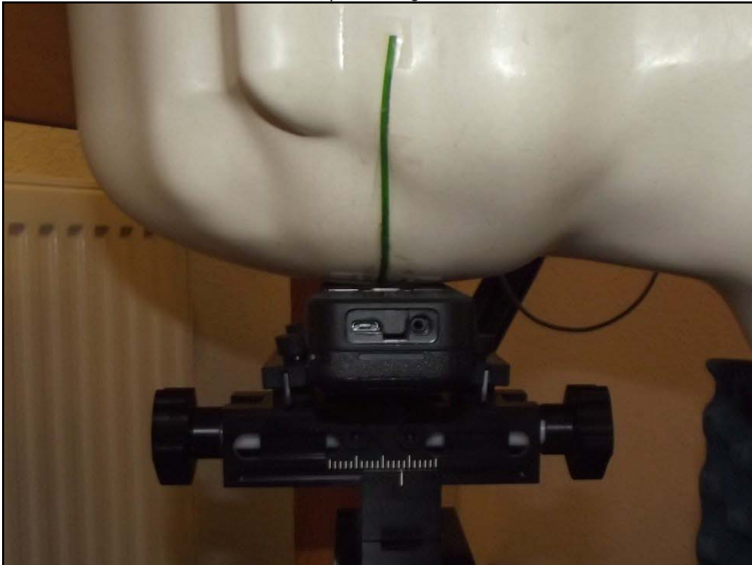
Photo 18: Test position right hand touched
