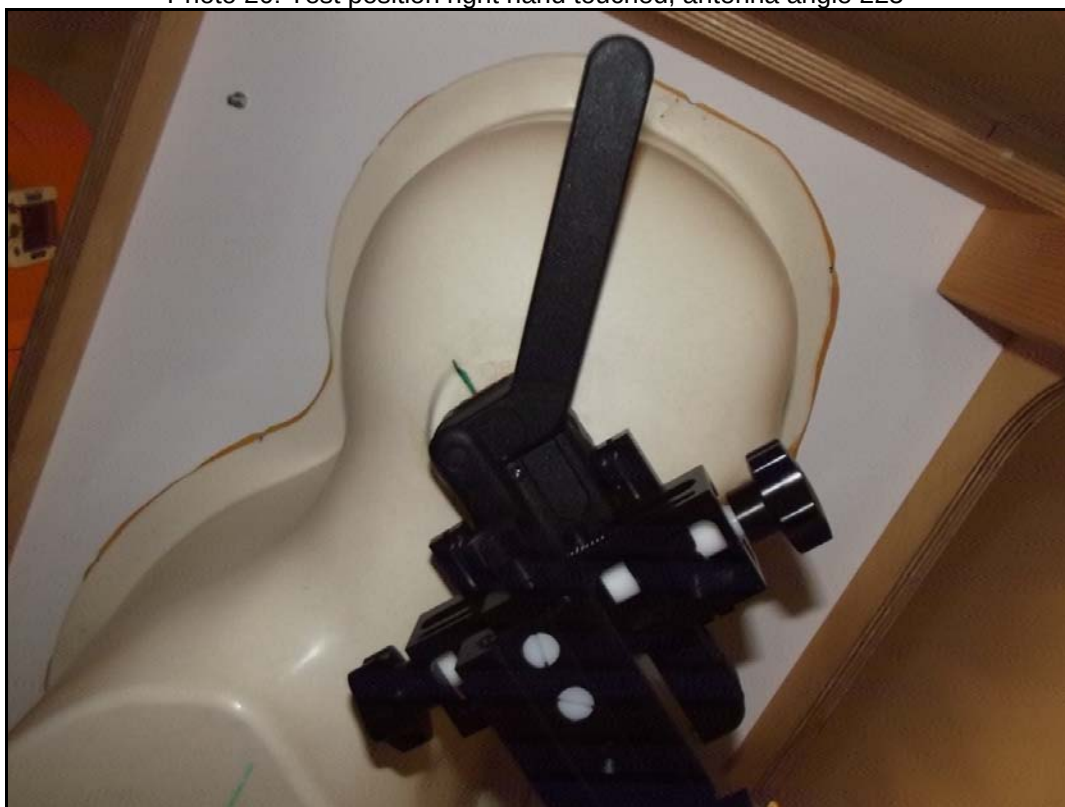
Photo 20: Test position right hand touched, antenna angle 225°
