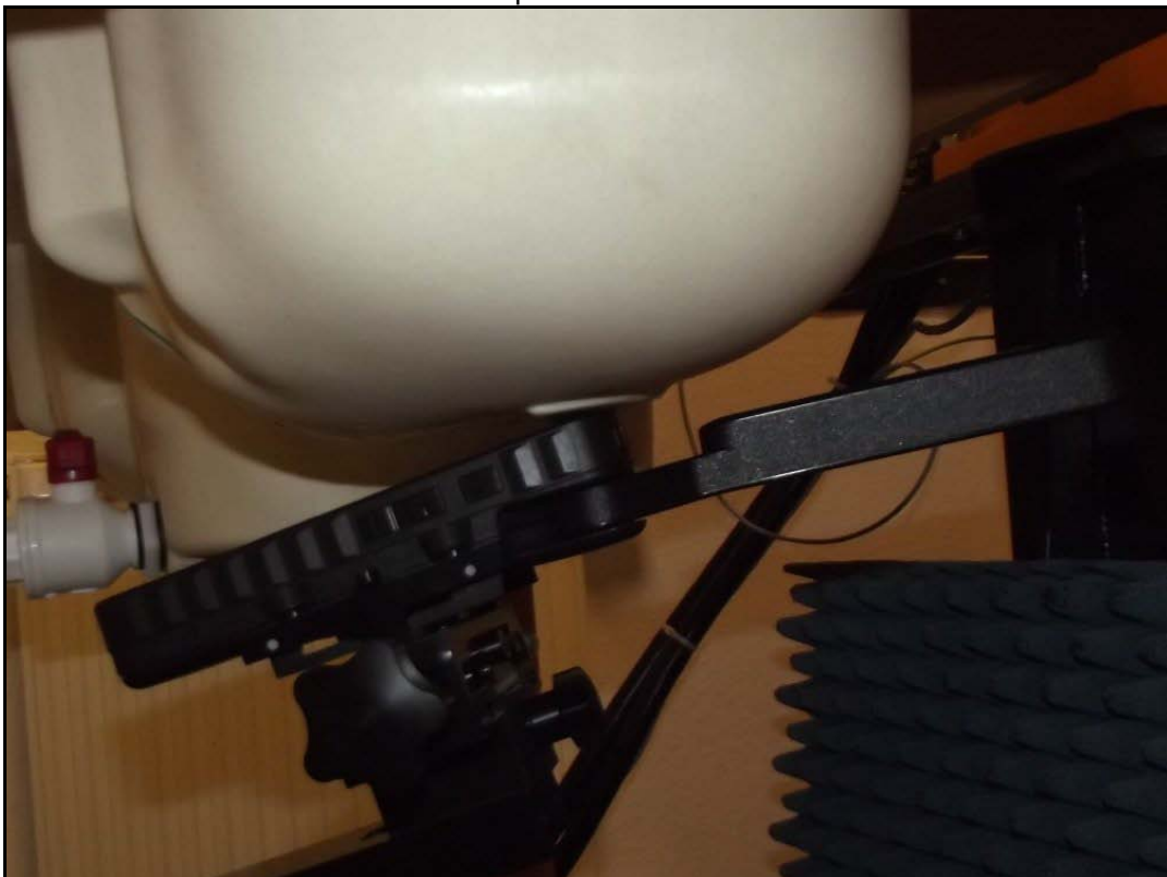
Photo 16: Test position left hand tilted 15°
