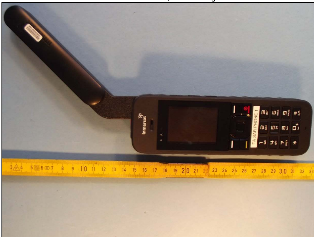
Photo 3: DUT - front view, antenna angle 135°
