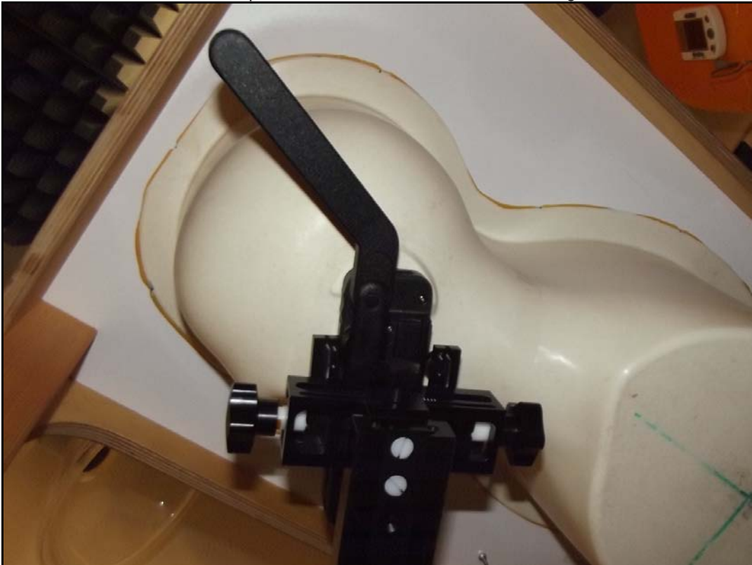
Photo 14: Test position left hand touched, antenna angle 180°
