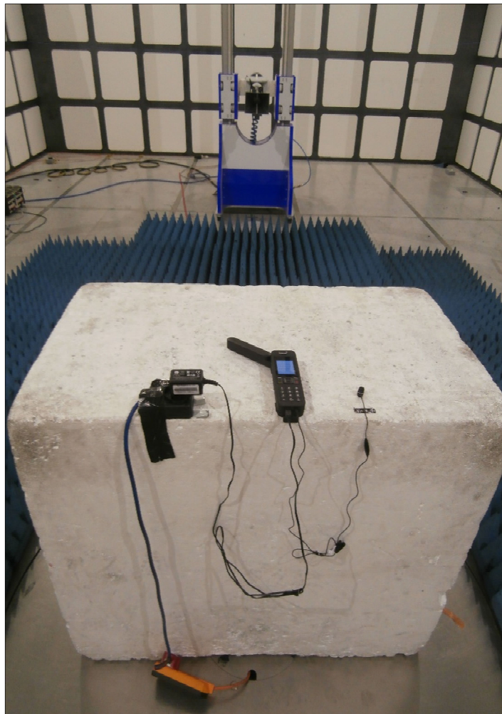
Figure 27 - Test Setup - 1 GHz to 18 GHz - X Orientation
