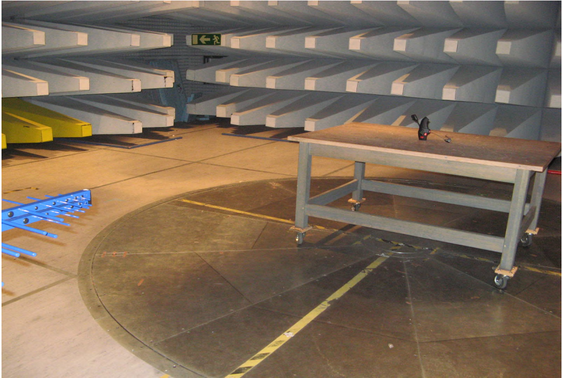
Photo 4.8.1 Test setup regarding measurement of spurious emission.
