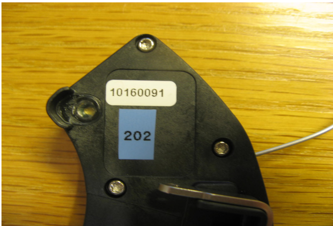
Photo 2.1.3 Photo of the tested object, unit 202, with a soldered SMA coaxial connector for conducted tests.
