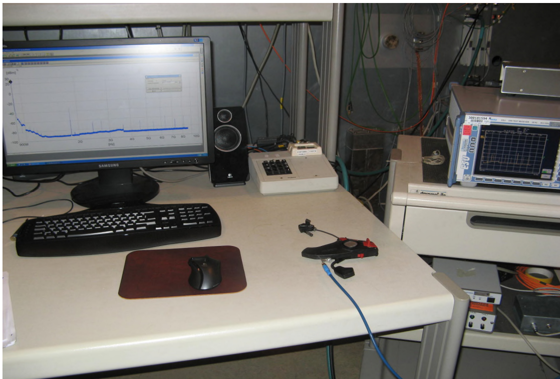
Photo 4.7.1 Test setup regarding measurement of conducted spurious emission.
