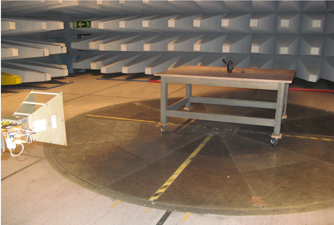
Photo 3.1.2 Test setup regarding spurious emission measurements.
