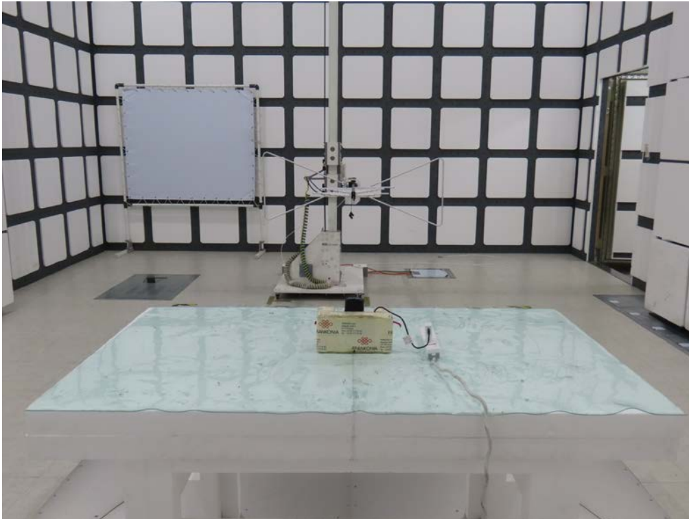
Set Up Photo of Conducted Emission EMI Mode 1
