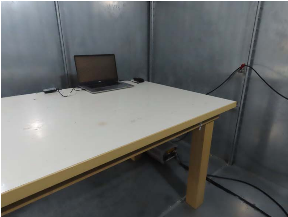
Set Up Photo of Conducted Emission EMI Mode 1
