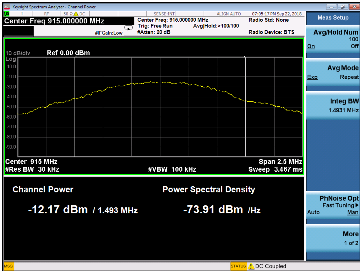
Low Data Rate Fundamental Emission Output Power
