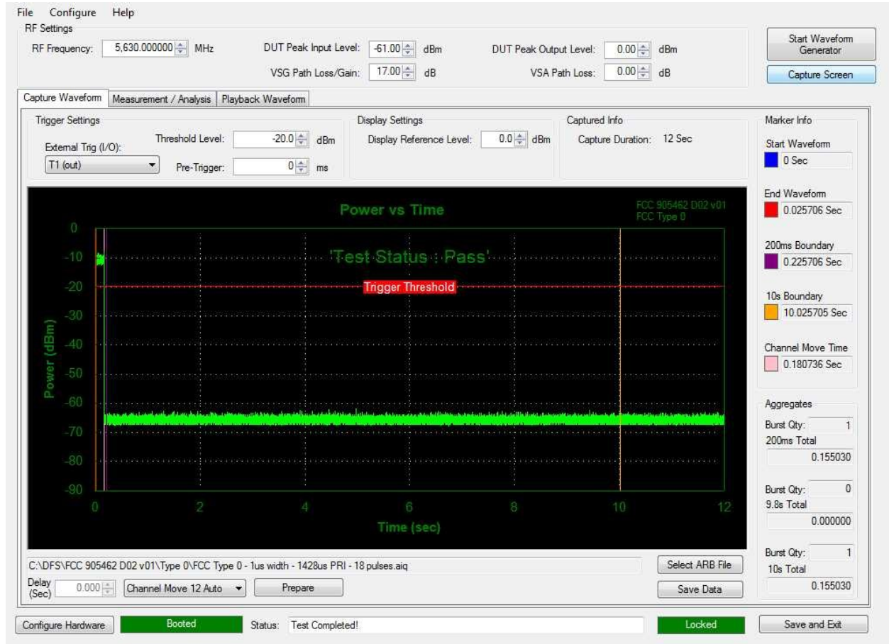
5630 MHz Overall Power vs Time Display, showing 10 seconds observation time
