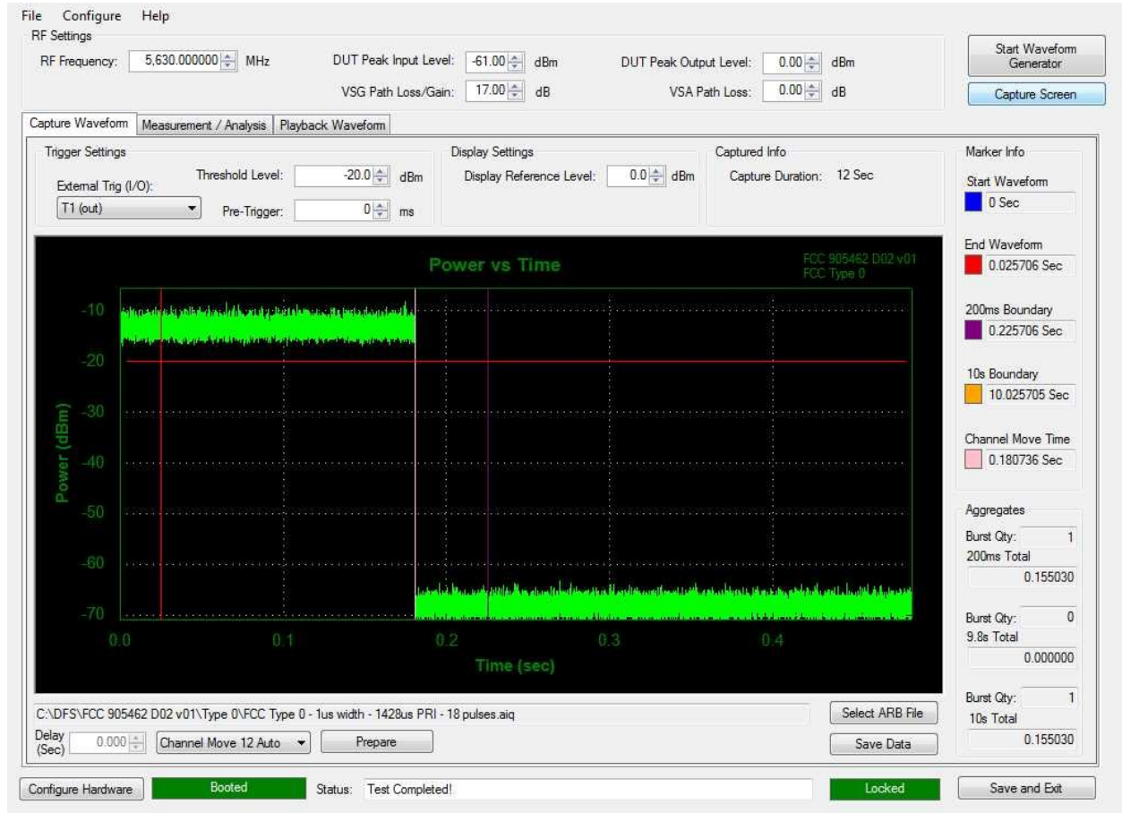
5630 MHz Zoomed In Overall Power vs Time Display, showing Channel Move Time (Pink), end of Radar Burst (Red) and the 200 ms boundary (Purple)
