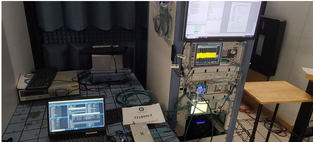
FCC Part 15.247 Conducted Test Setup
