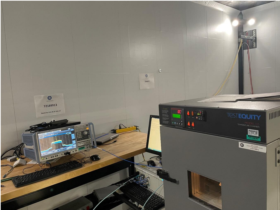
Frequency Stability Test Setup
