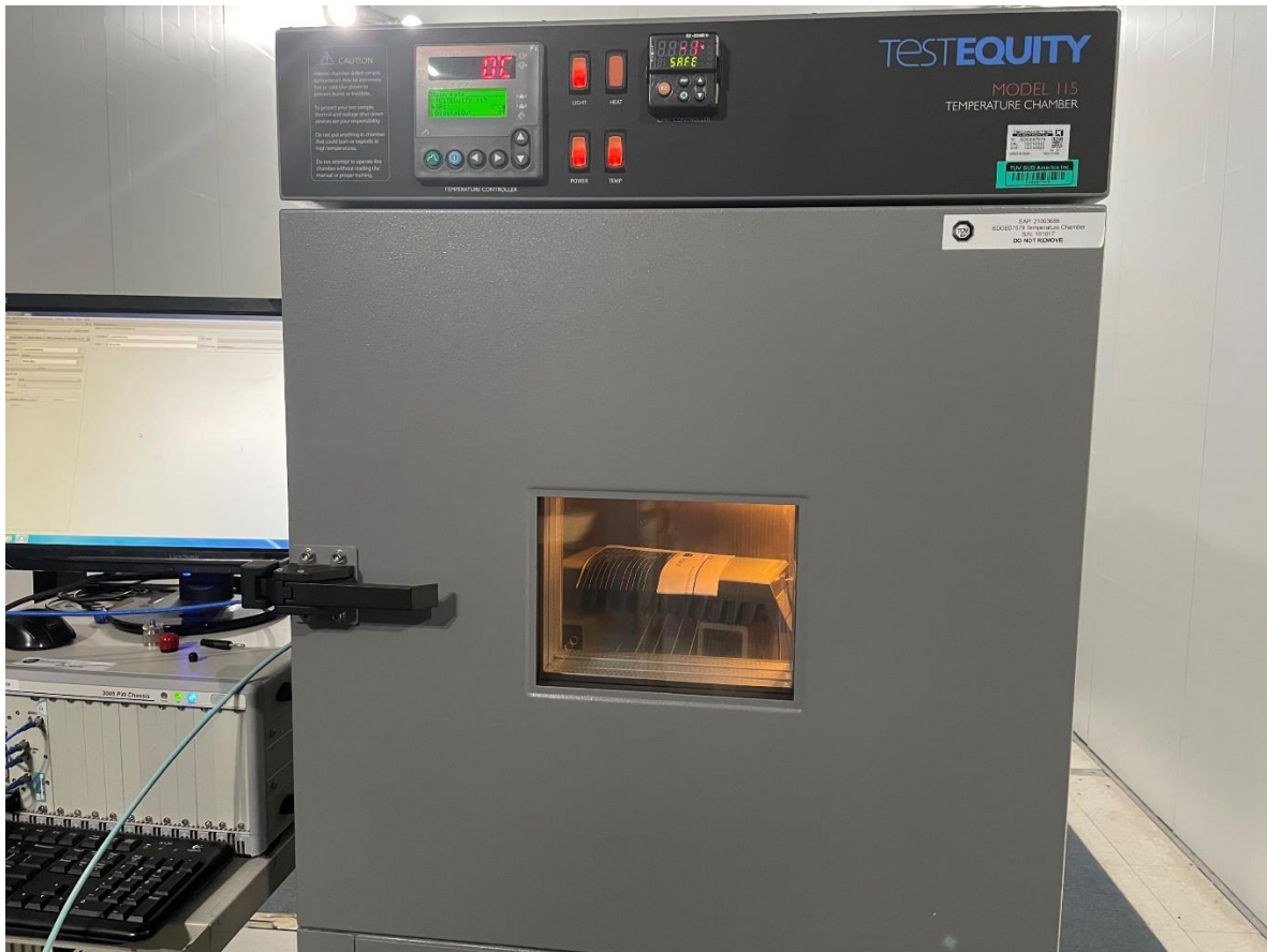
Frequency Stability Test Setup
