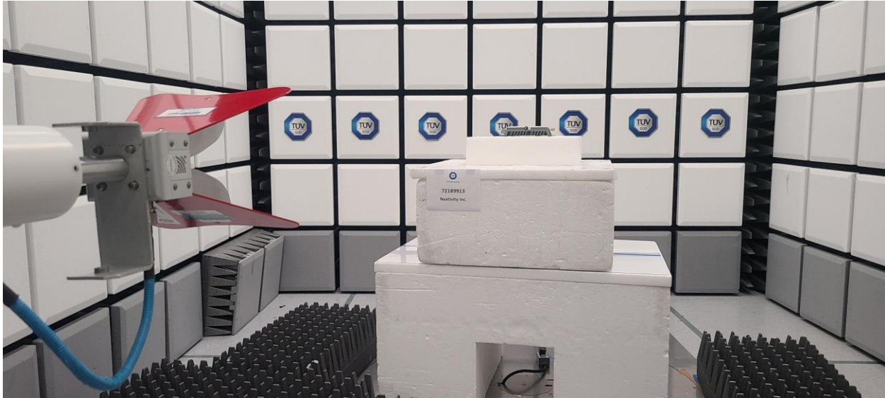
FCC Part 15.247 Radiated Emissions Test Setup (1 GHz to 18 GHz)
