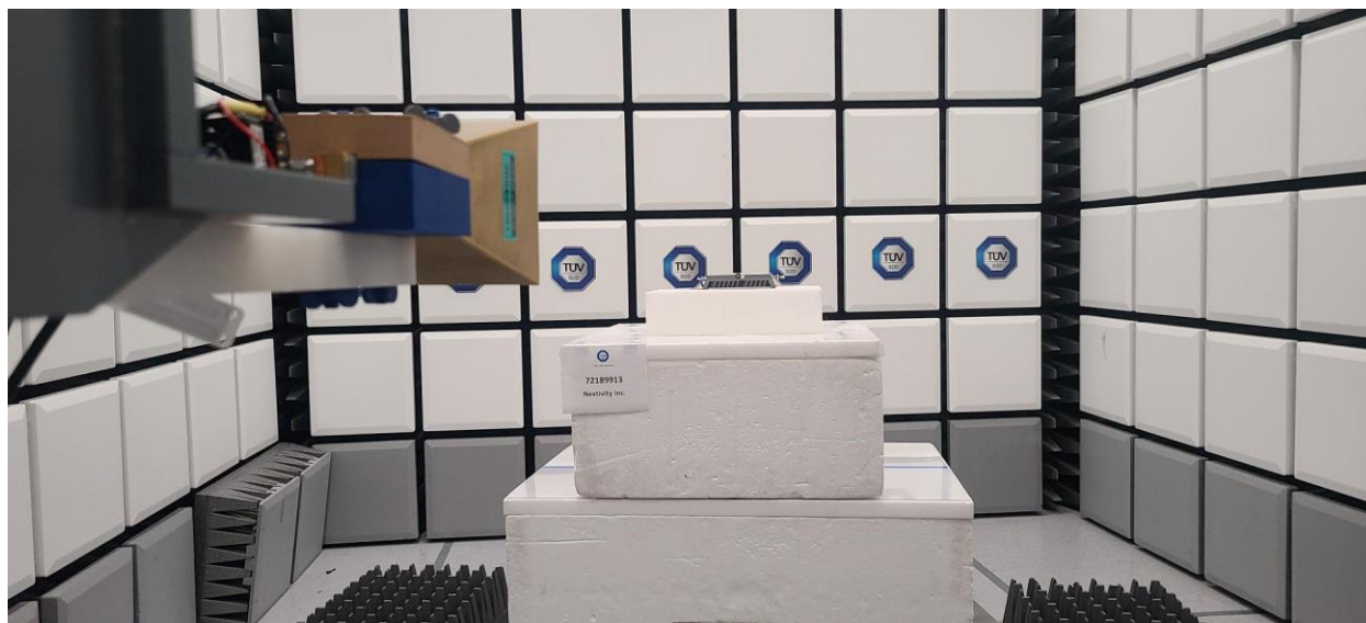
FCC Part 15.247 Radiated Emissions Test Setup (1 GHz to 26 GHz)
