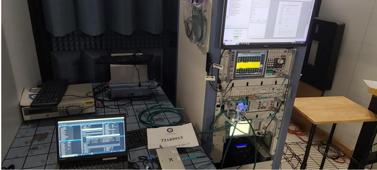
FCC Part 15.247 Conducted Test Setup
