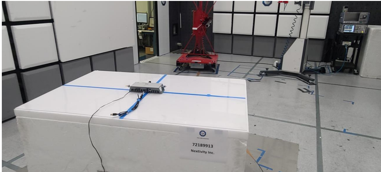
FCC Part 15.247 Radiated Emissions Test Setup (30 MHz to 1 GHz)
