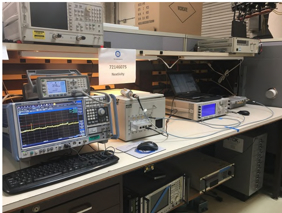
Conducted RF Testing
