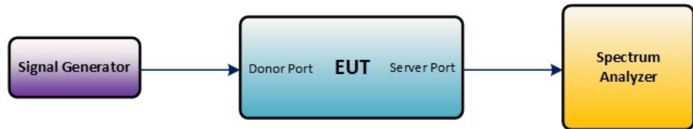
Figure 3 – Downlink test configuration in EUT test mode
