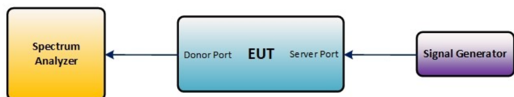
Figure 2 – Uplink test configuration in EUT test mode
