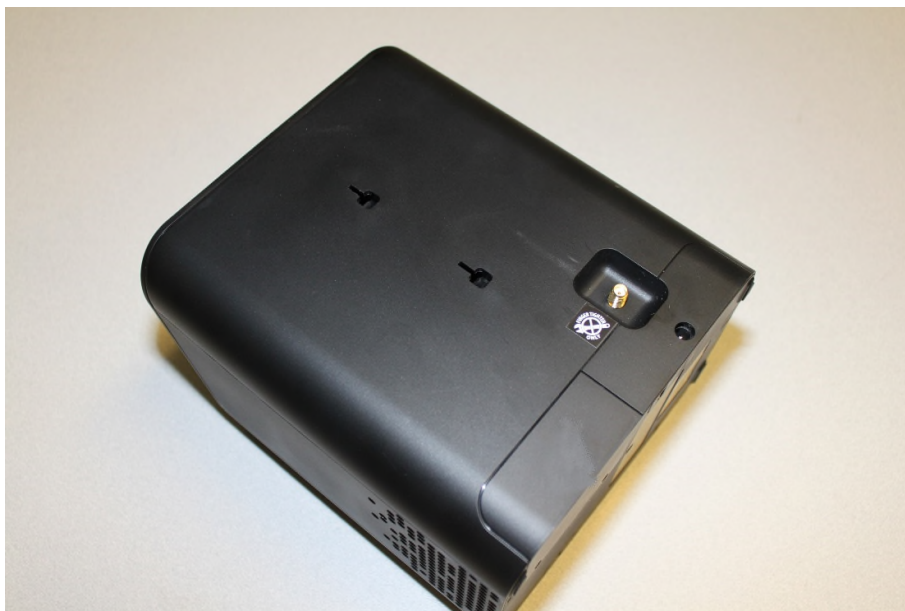
EUT (Network Unit) showing additional external antenna port subject to C2PC
