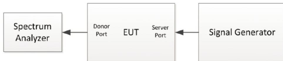
Figure 2: Uplink Test Configuration in Test Mode
