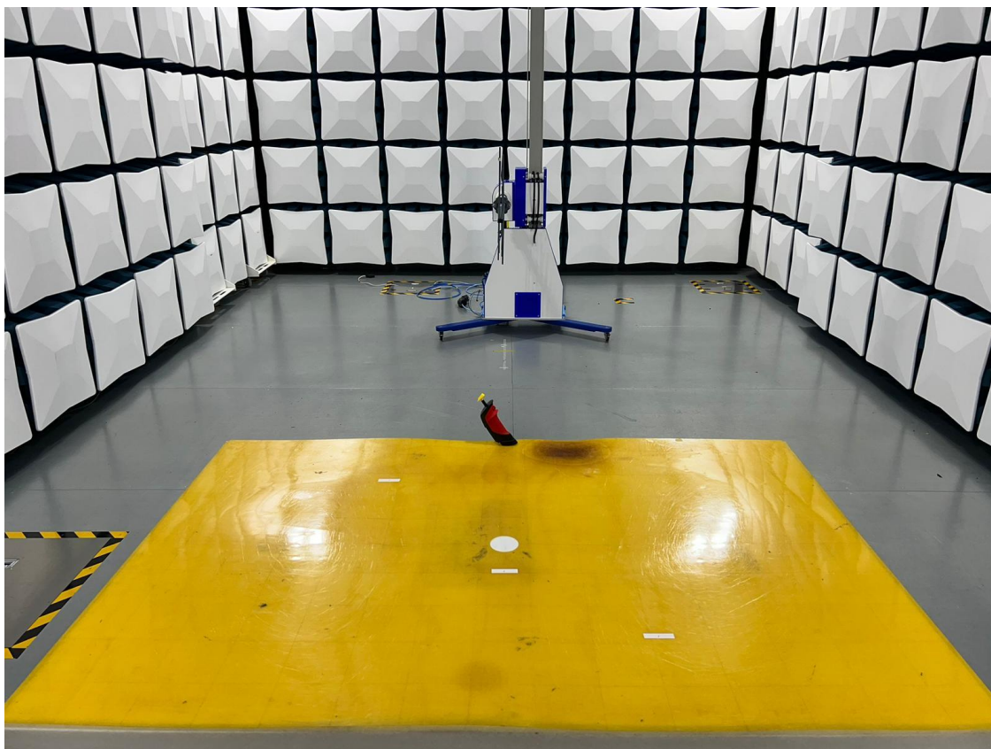
Set-up for Radiated Emission (200-1000MHz)
