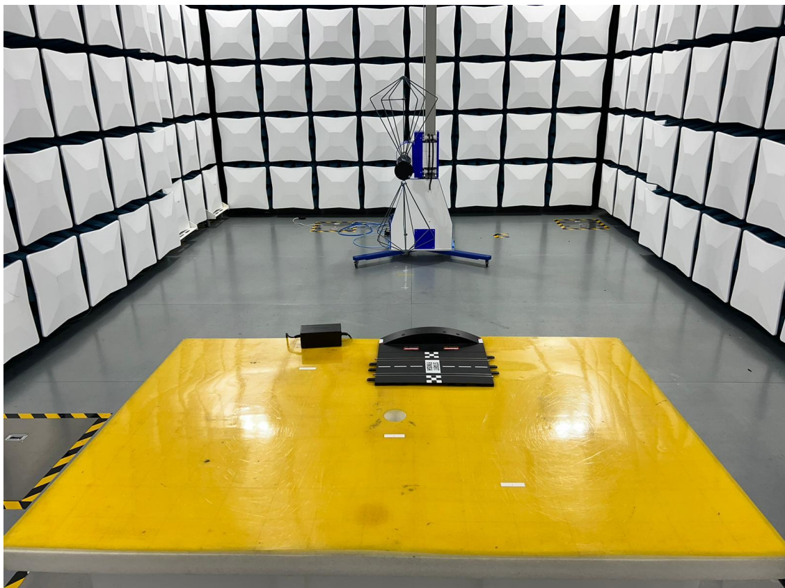
Set-up for Radiated Emission (30-200MHz)
