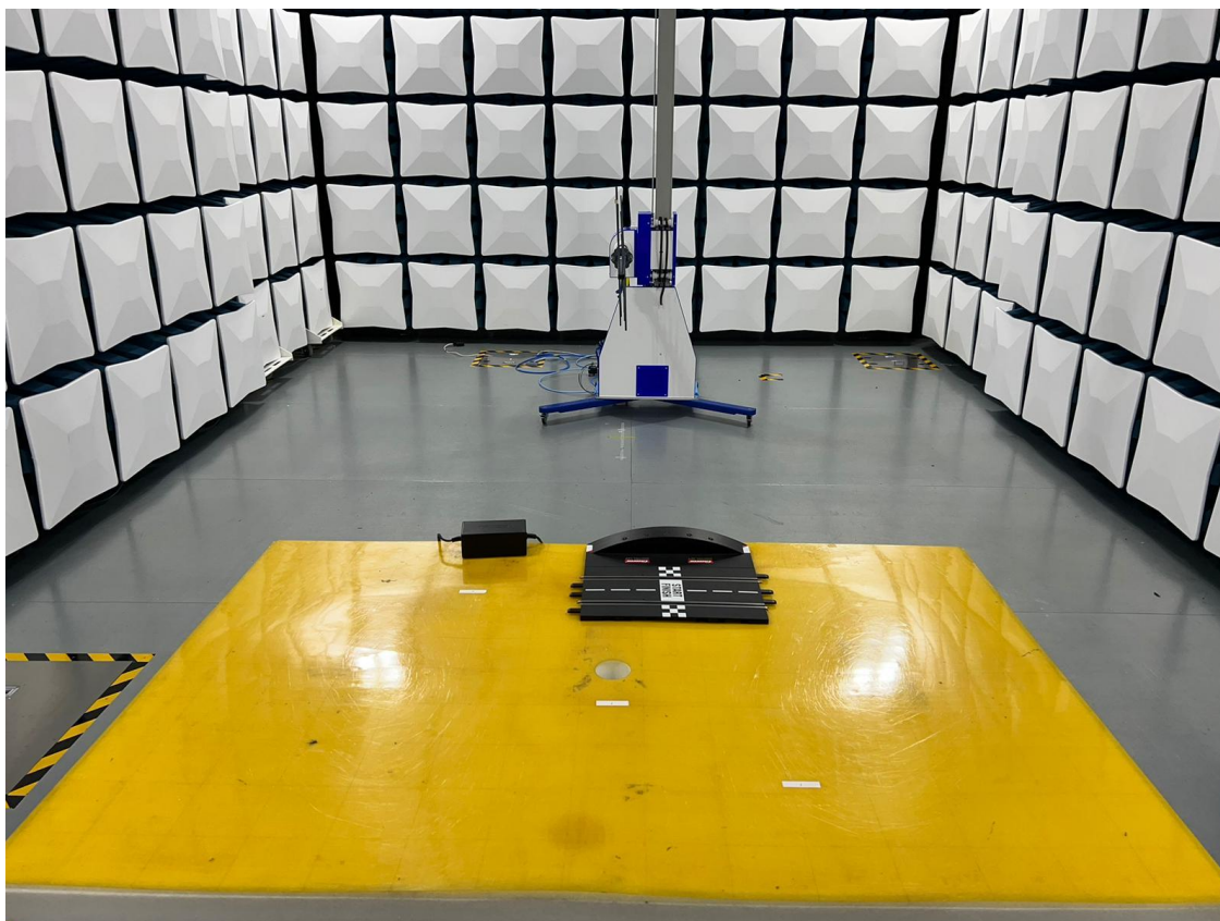
Set-up for Radiated Emission (200-1000MHz)
