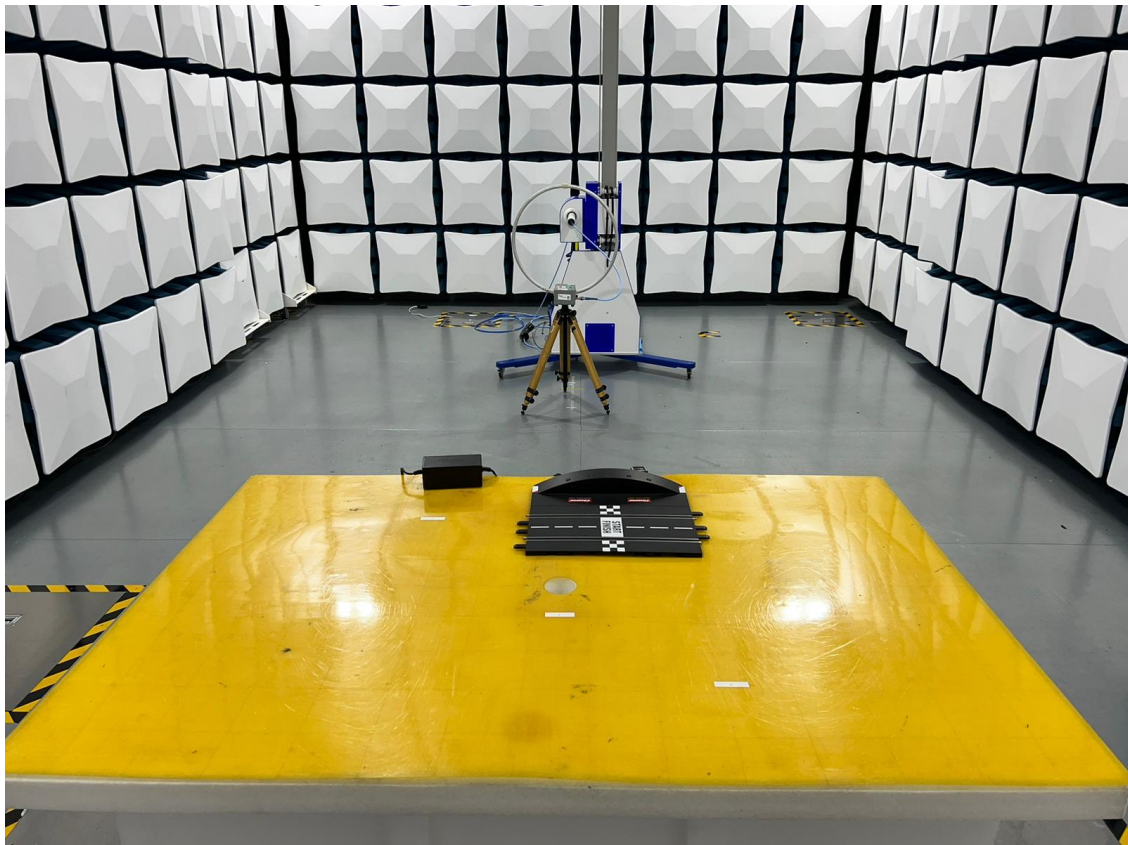
Set-up for Radiated Emission (9k-30MHz)
