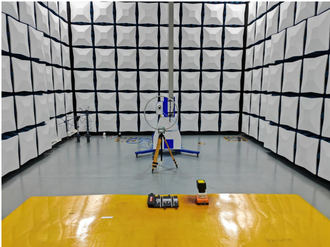
Set-up for Radiated Emission (9k-30MHz)
