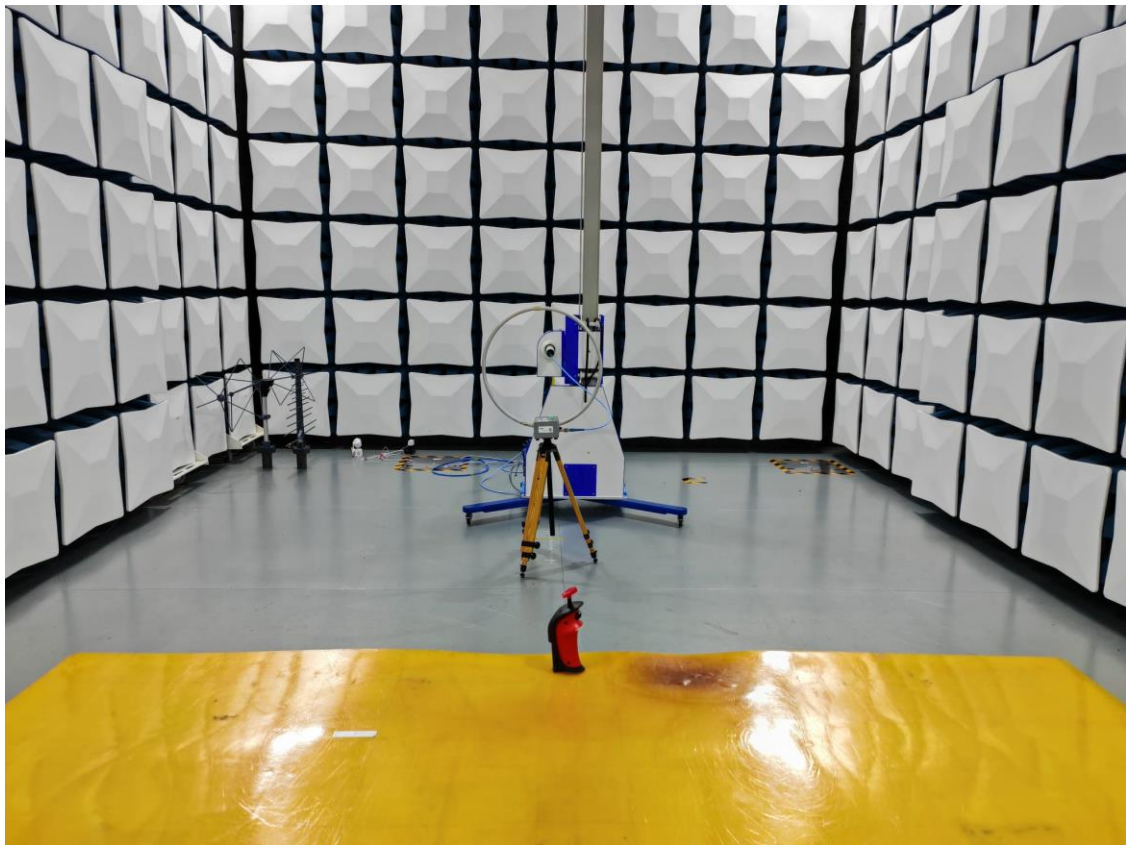
Set-up for Radiated Emission (9k-30MHz)
