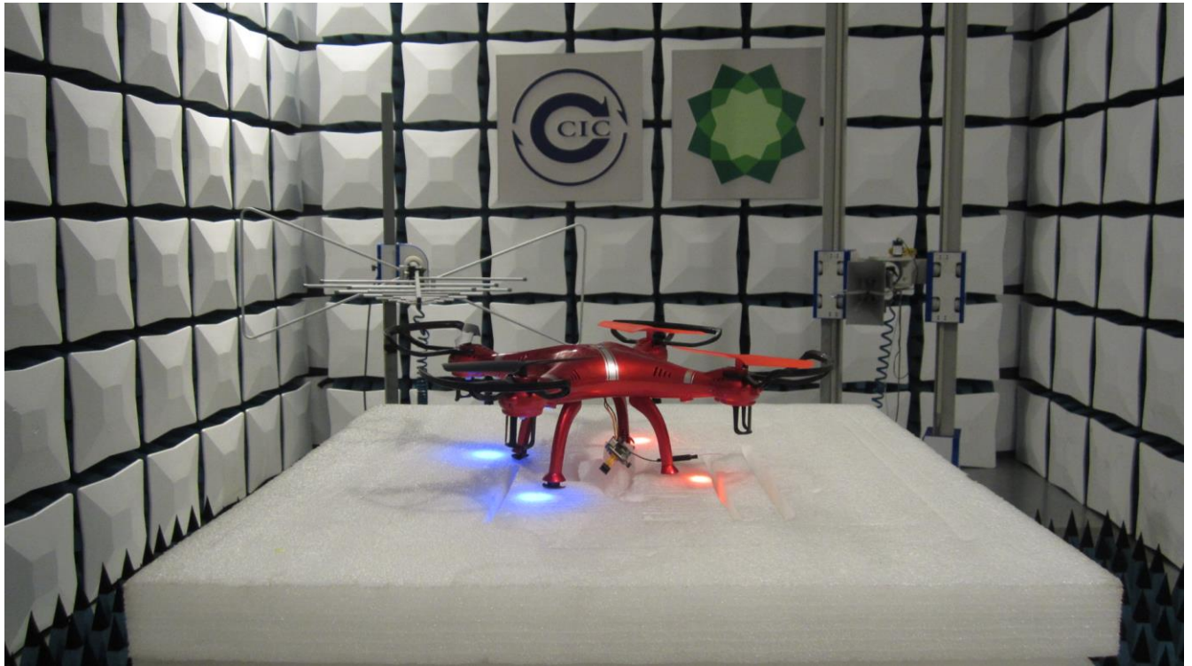
Set-up for Radiated Emission above 1GHz measurement
